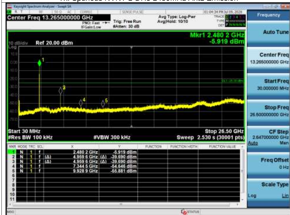
Tx. Spurious NVNT 1-DH5 2480MHz Ant1 Emission
