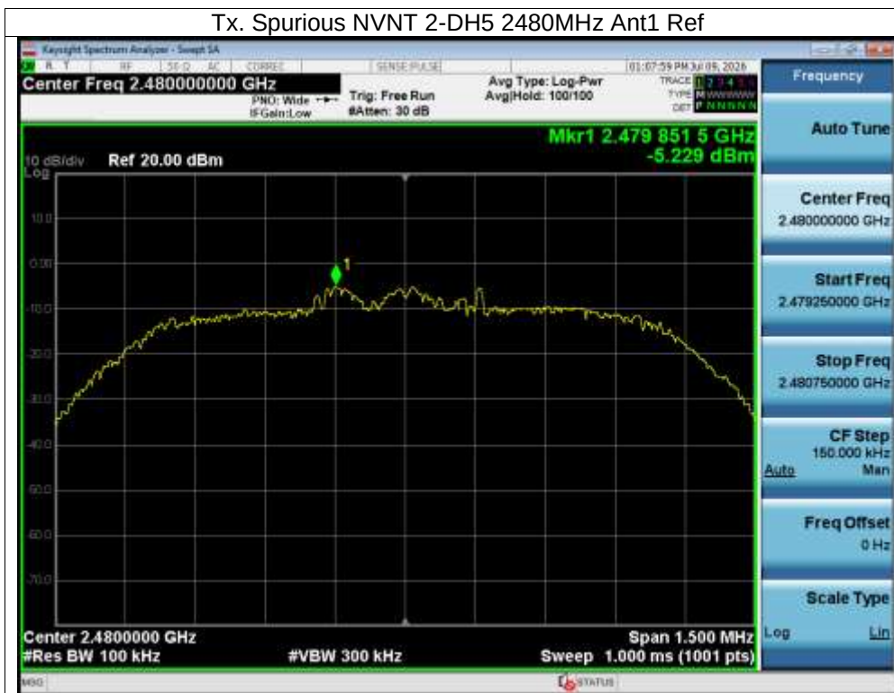
Tx. Spurious NVNT 2-DH5 2480MHz Ant1 Emission
