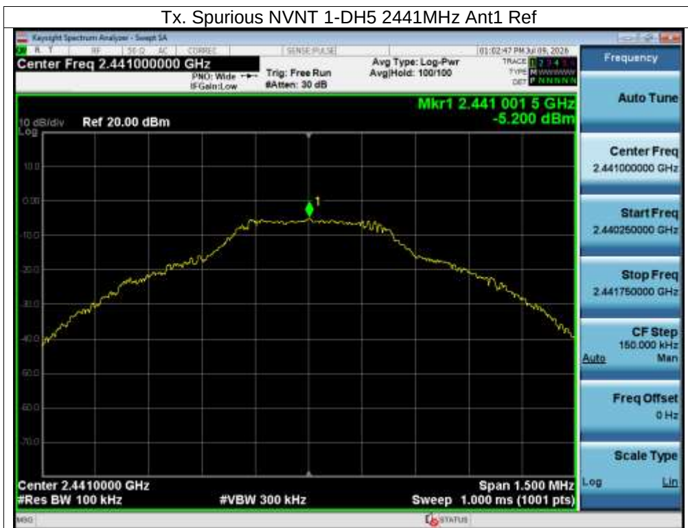
Tx. Spurious NVNT 1-DH5 2441MHz Ant1 Emission
