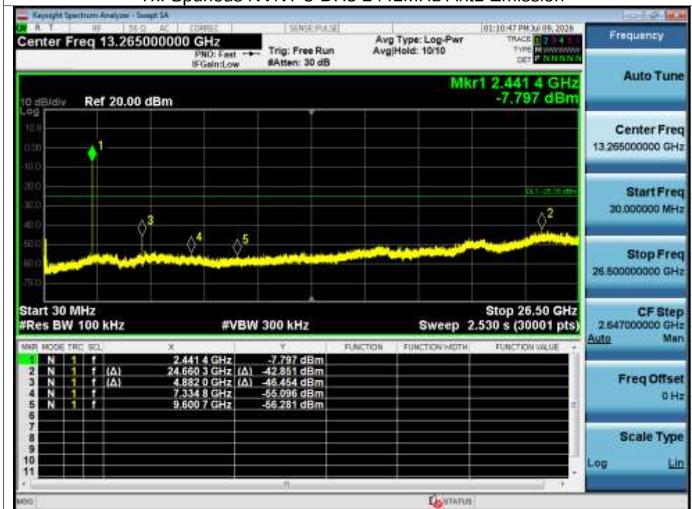
Tx. Spurious NVNT 3-DH5 2441MHz Ant1 Emission
