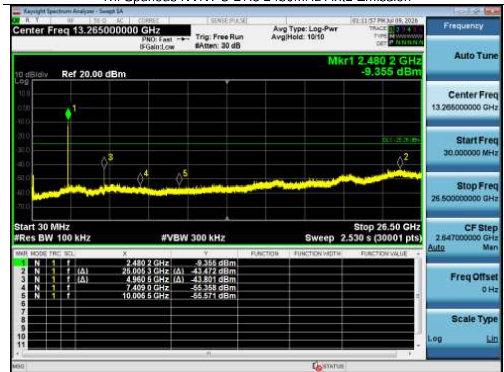
Tx. Spurious NVNT 3-DH5 2480MHz Ant1 Emission
