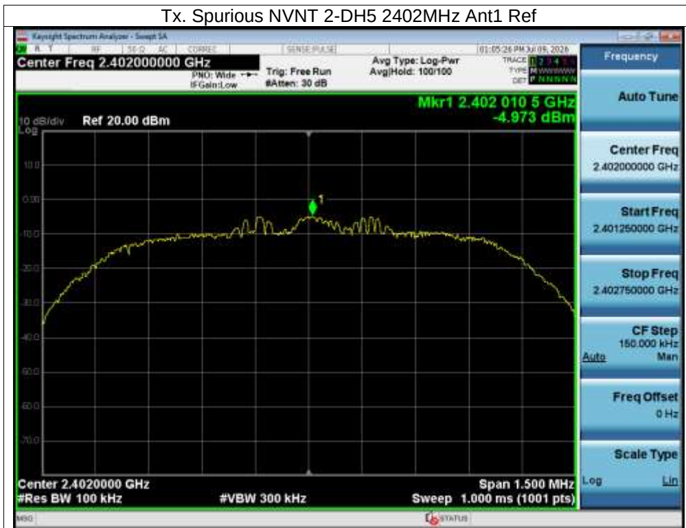
Tx. Spurious NVNT 2-DH5 2402MHz Ant1 Emission
