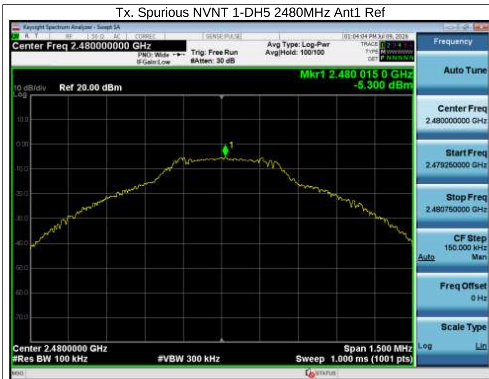
Tx. Spurious NVNT 1-DH5 2480MHz Ant1 Emission
