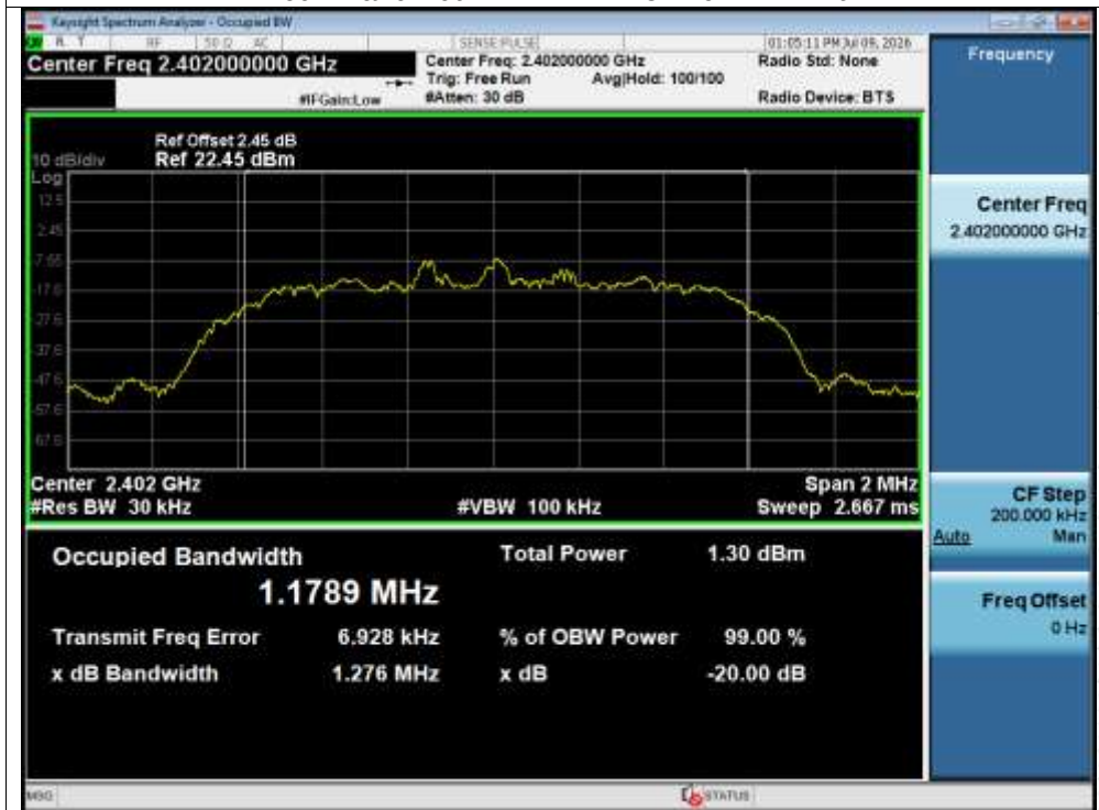
-20dB Bandwidth NVNT 2-DH5 2402MHz Ant1
