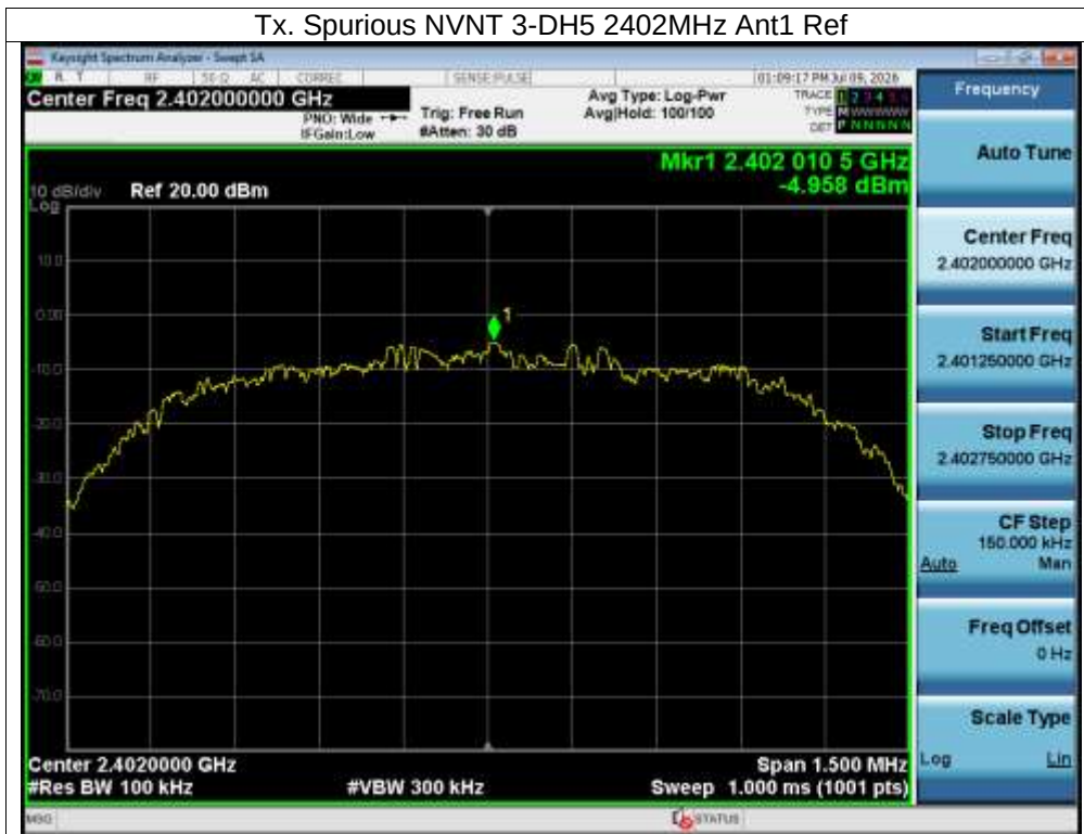
Tx. Spurious NVNT 3-DH5 2402MHz Ant1 Emission
