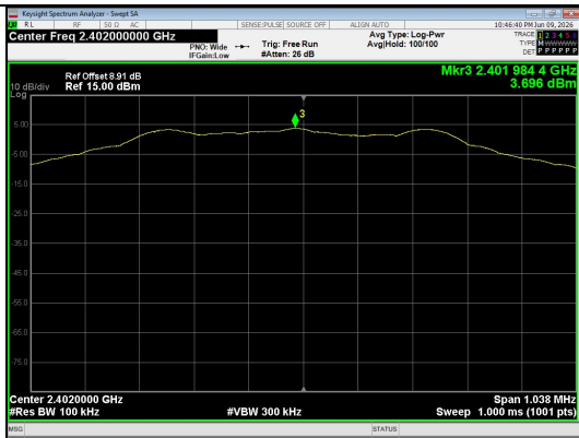
In-Band Reference Level BLE 1M_Channel 0
