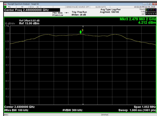
In-Band Reference Level BLE 1M_Channel 39
