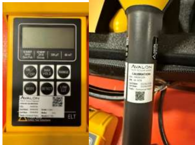
Calibrated Narda ELT-400 Meter and Probe Utilized for Testing
