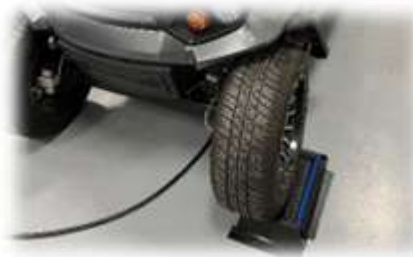
Figure 8: Vehicle positioning off edge of wheel guide for purposeful misalignment
