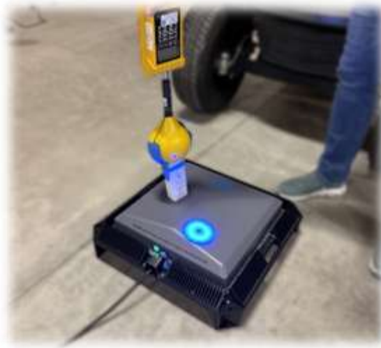
Figure 11: Field Probe Setup for Standby Measurements
