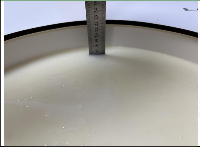
Photo 1: Tissue Simulant Liquid for Head 700-3000Mhz
