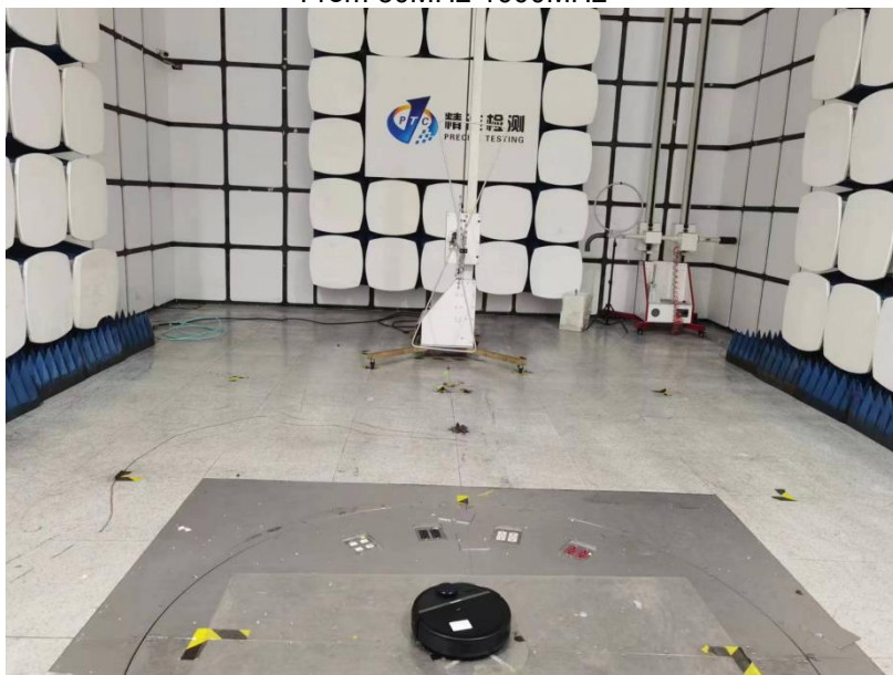
Radiated Spurious Emissions From 30MHz-1000MHz
