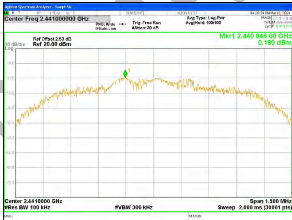
Tx. Spurious NVNT 2-DH1 2441MHz Ant1 Emission
