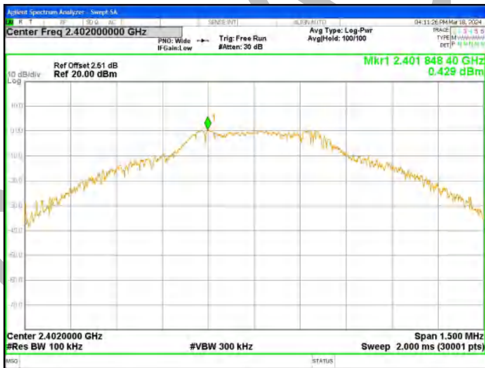
Tx. Spurious NVNT 1-DH1 2402MHz Ant1 Emission
