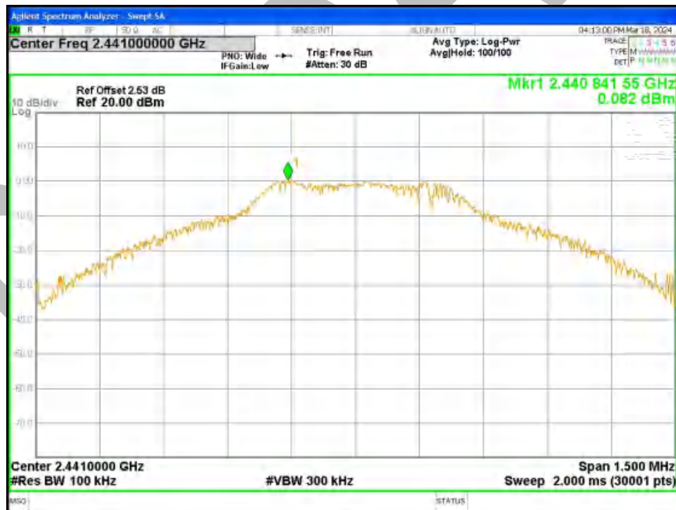
Tx. Spurious NVNT 1-DH1 2441MHz Ant1 Emission
