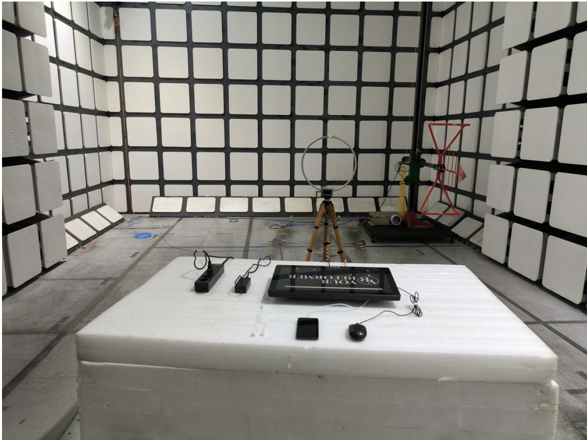
Radiated Emissions View (Below 1GHz)
