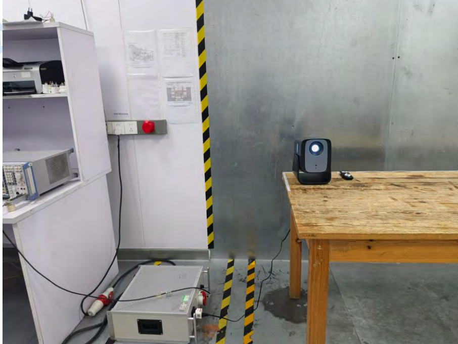
Conducted Emission at AC power line
