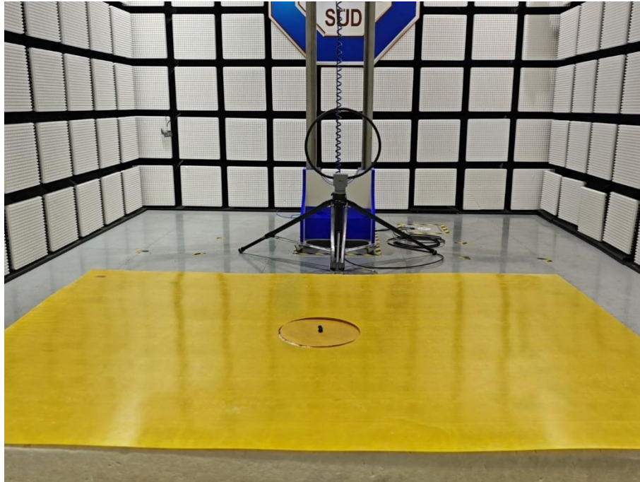
9kHz-30MHz RSE Setup
