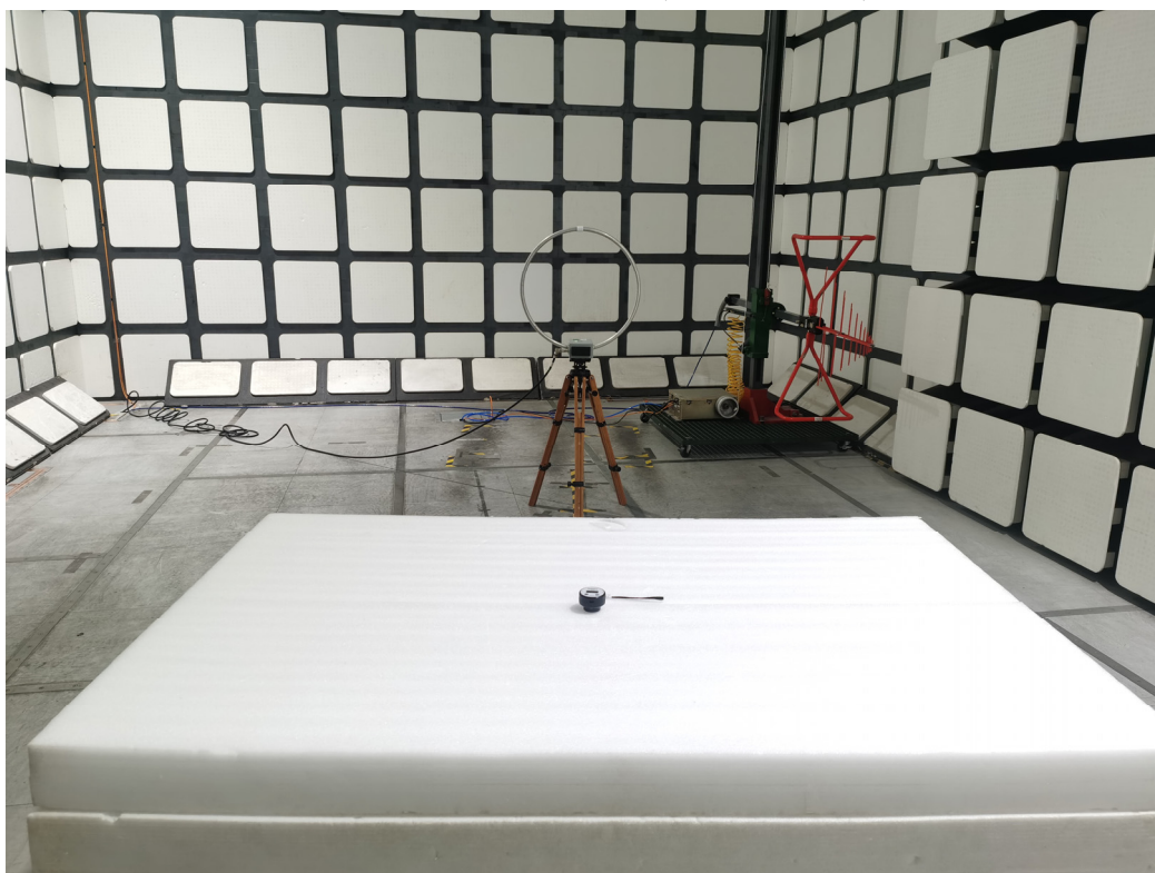
Radiated Emissions View (9kHz- 30MHz)
