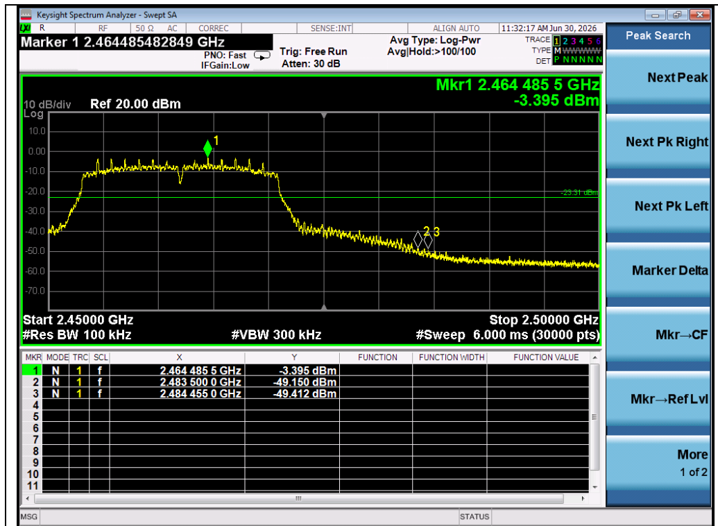
Test_Graph_802.11n20_ANT1_2462_MCS0_Higher Band Edge Emissions
