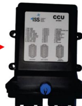
CCU placed behind the cab
