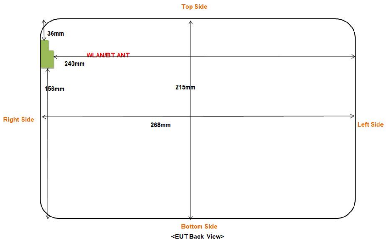
Fig 7.2 Block Diagram for EUT Antenna Position
