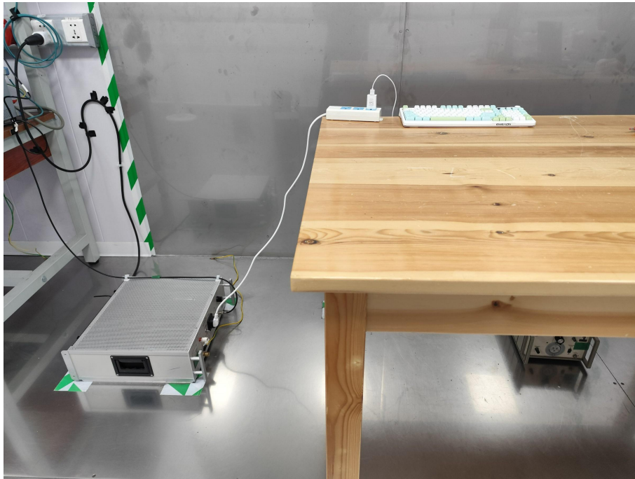
Conducted Emission at AC power line
