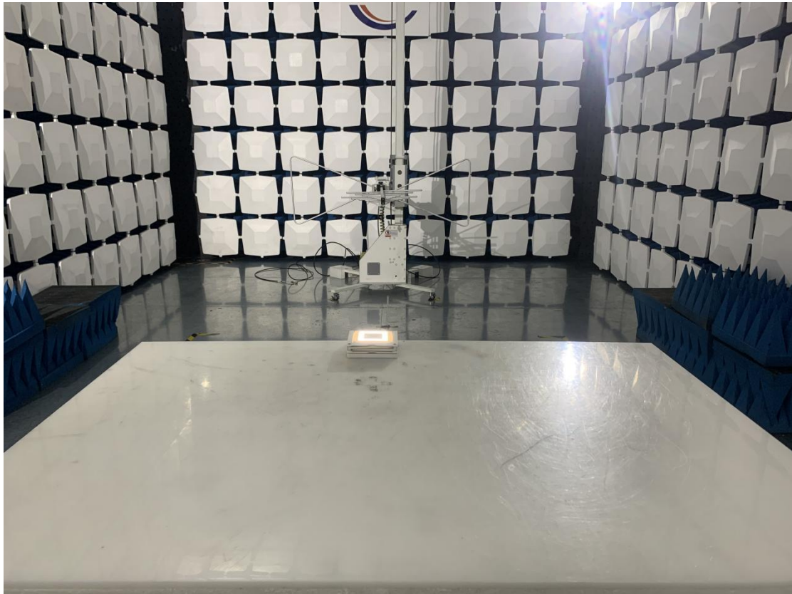
Above 1GHz for radiated emission test setup
