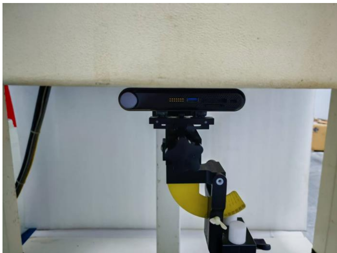
Fig-4.3 Rear Face of EUT with 0 cm Gap (Body Mode)
