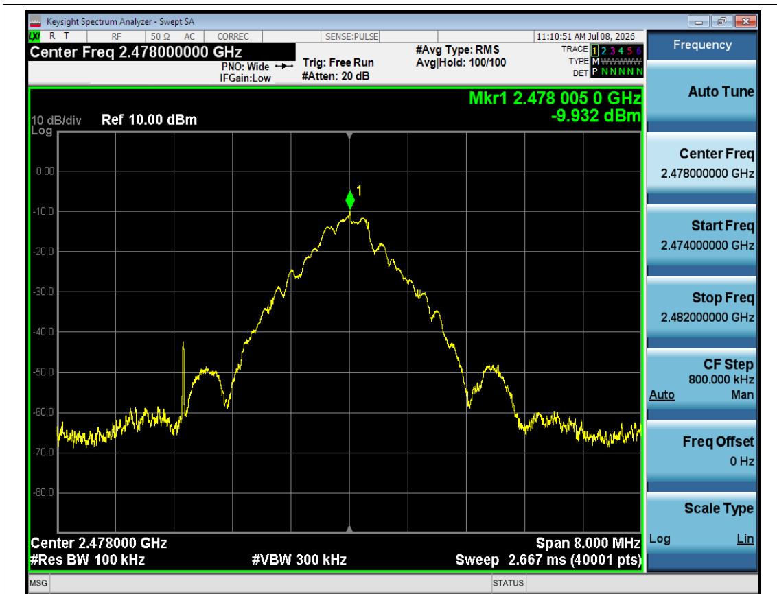
Tx. Spurious NVNT 2.4GHz 2M 2478MHz Ant1 Ref
