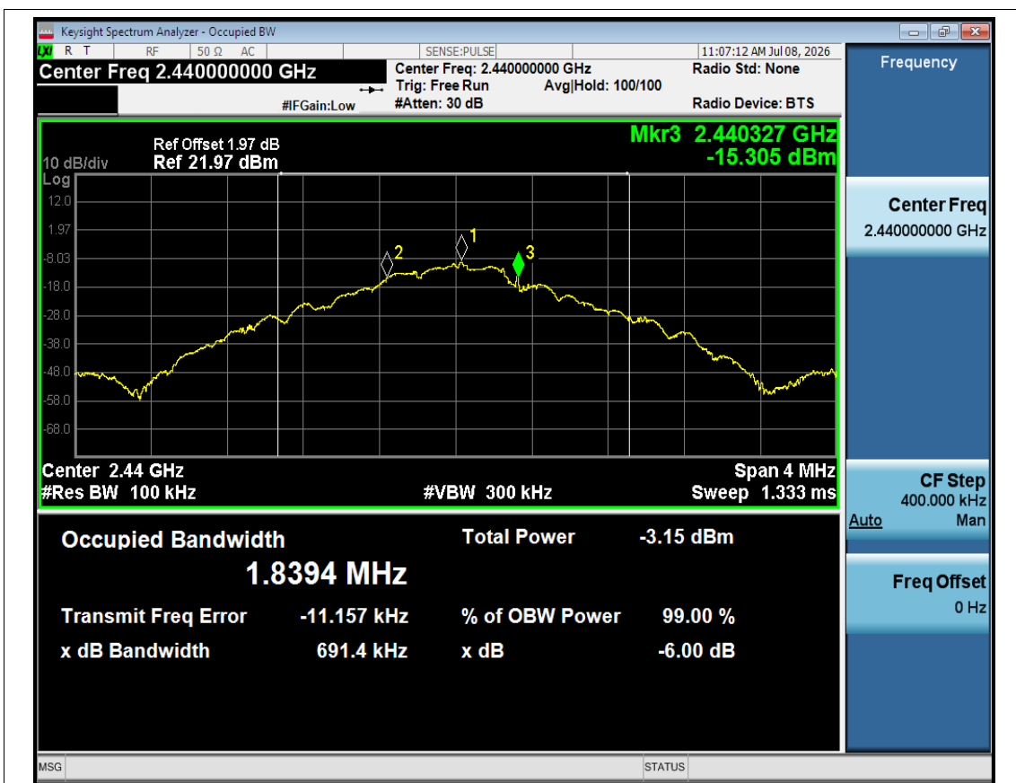
-6dB Bandwidth NVNT 2.4GHz 2M 2440MHz Ant1
