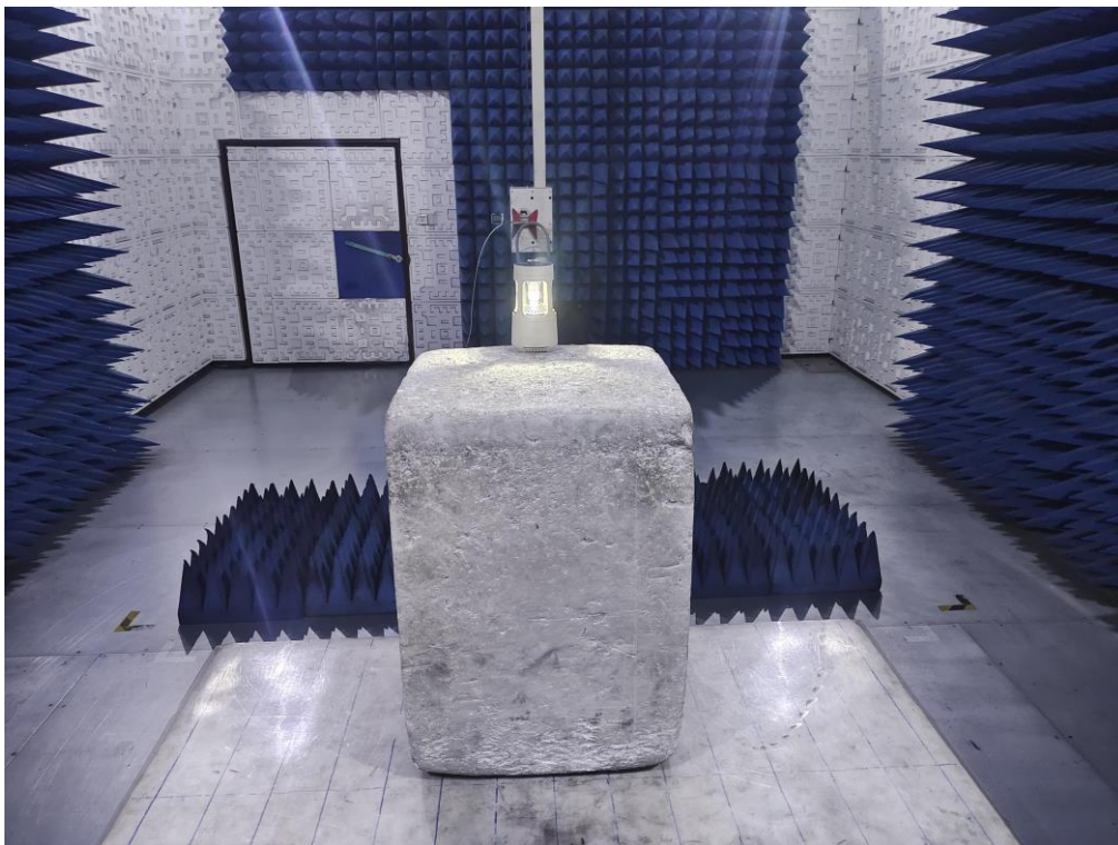
RADIATED EMISSION TEST SETUP ABOVE 1GHz
