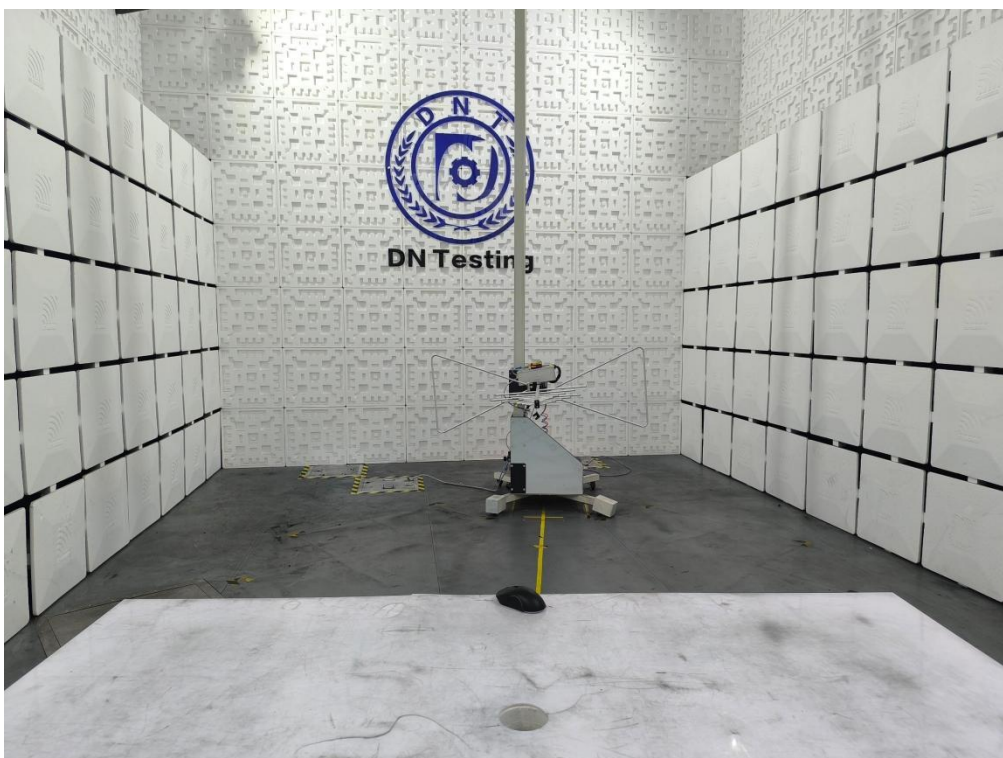
Radiated Emission Test View|(Below 1G)
