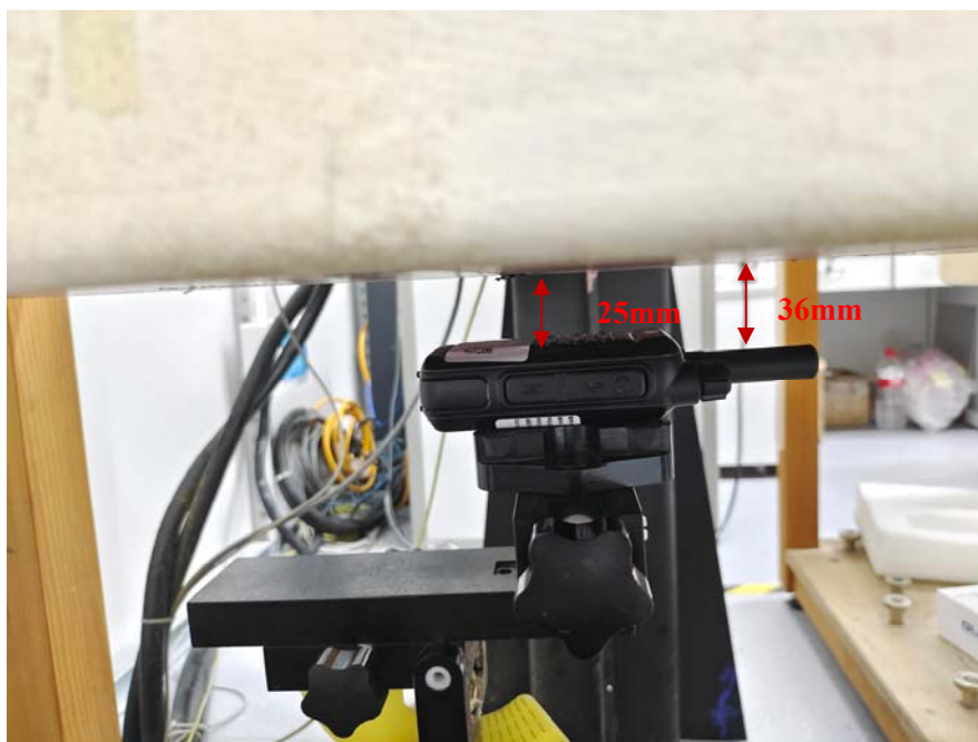
Face Up Setup Photo (25mm)
