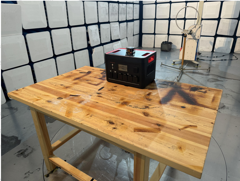
Photo of Radiation Emission Test (below 30MHz)
