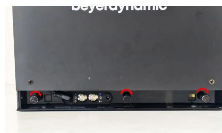
6.3.3 Rotate the screws to the right and tighten 3 screws
