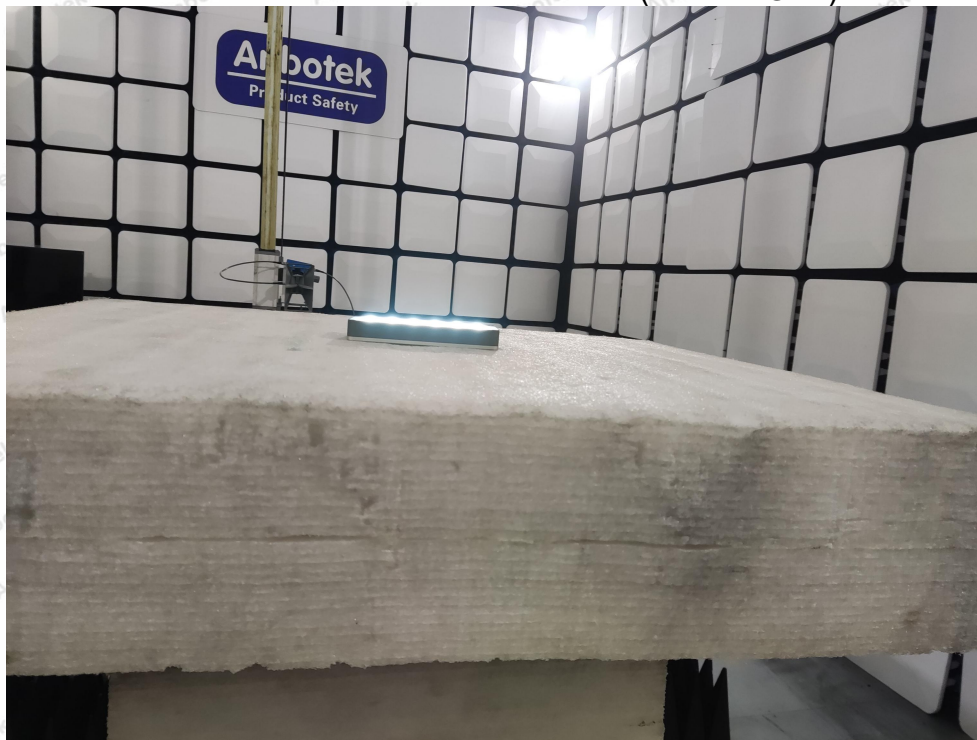
Photo of Radiation Emission Test (above 1GHz)
