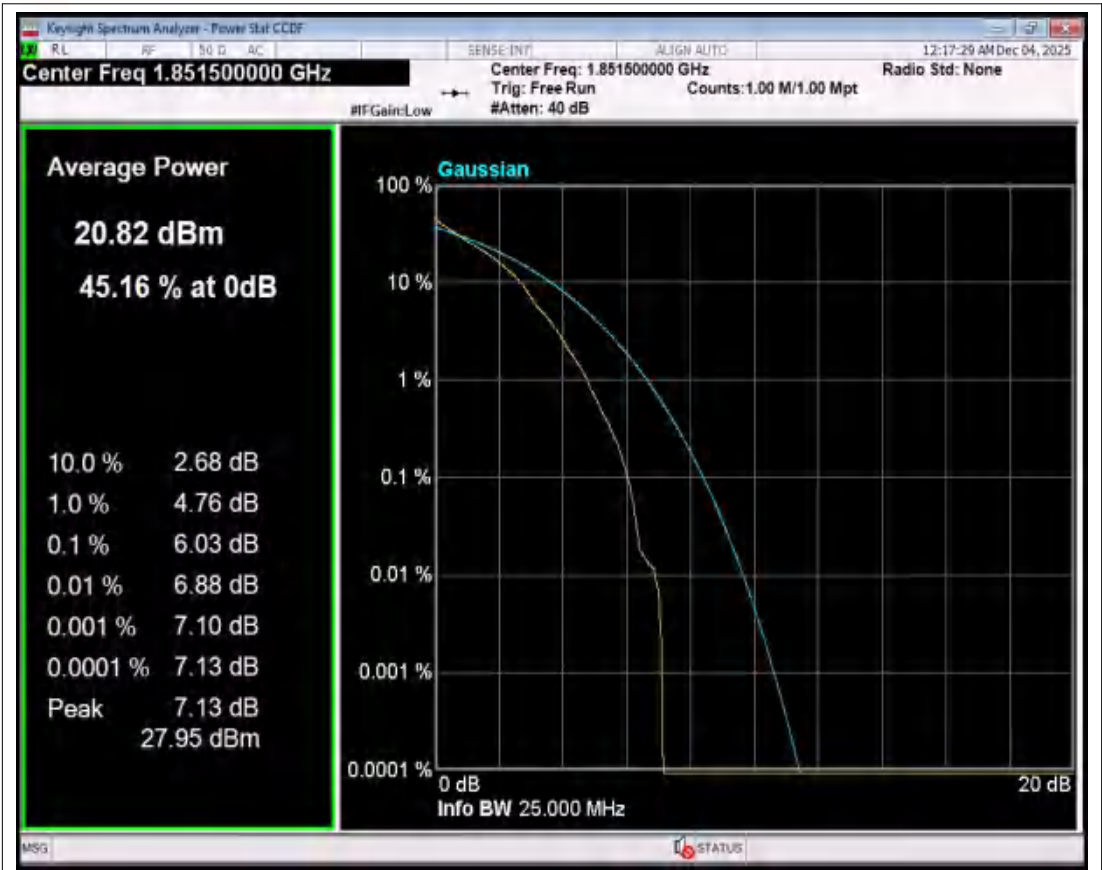
Band2 QPSK BW=3MHz Channel=18615 RB Size=1 Position=#0 NVNT
