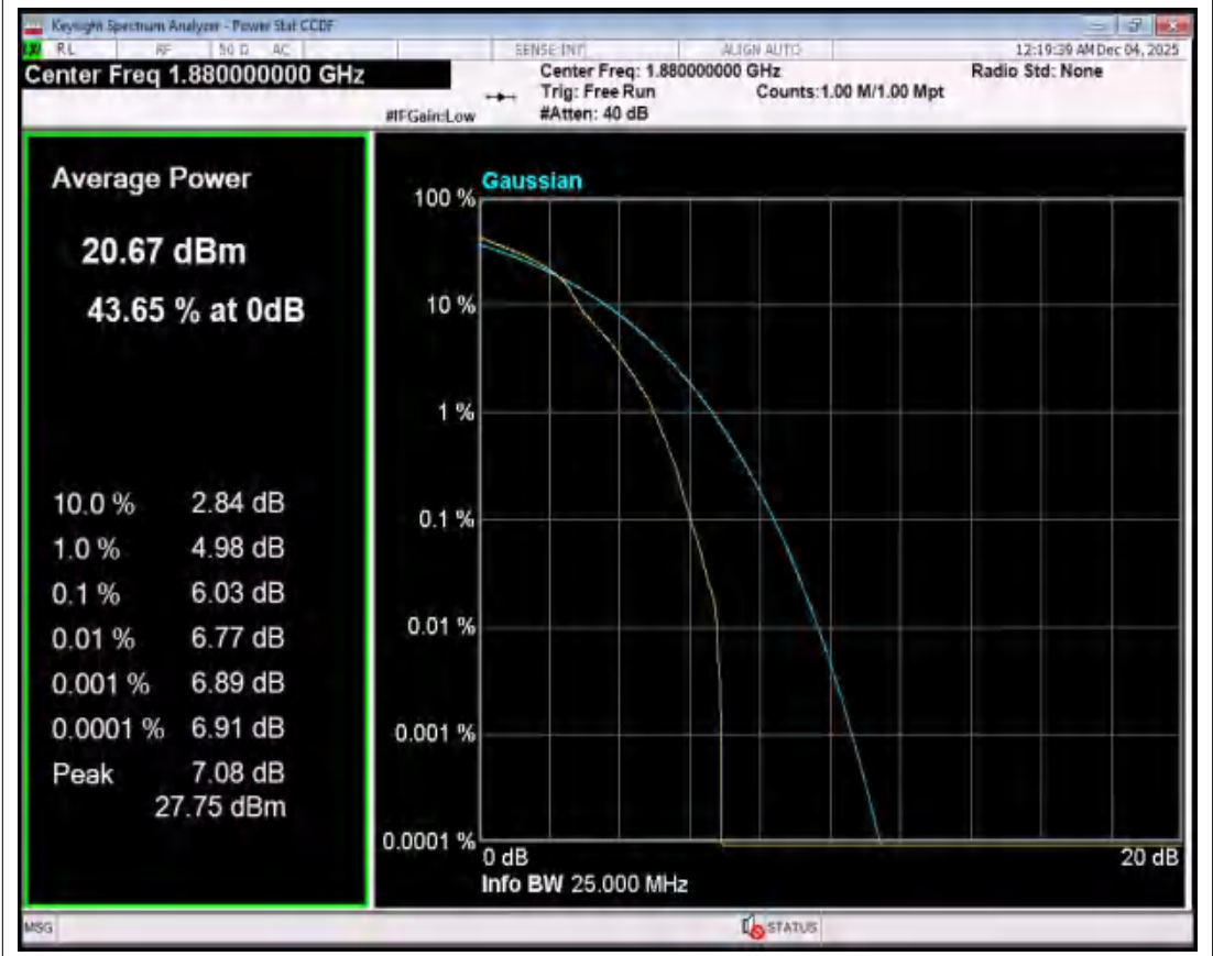
Band2 16QAM BW=20MHz Channel=18900 RB Size=1 Position=#0 NVNT
