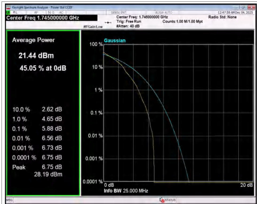
Band4 QPSK BW=20MHz Channel=20300 RB Size=1 Position=#0 NVNT
