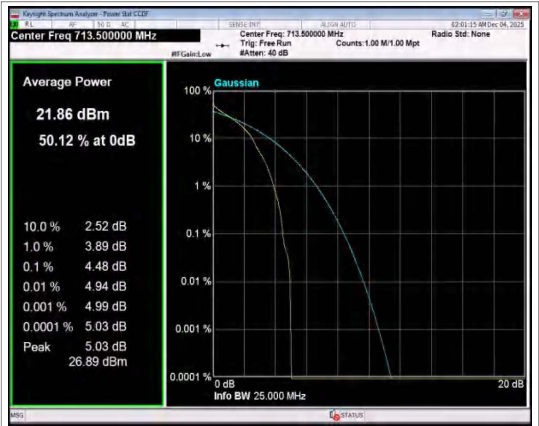
Band17 QPSK BW=5MHz Channel=23825 RB Size=1 Position=#0 NVNT
