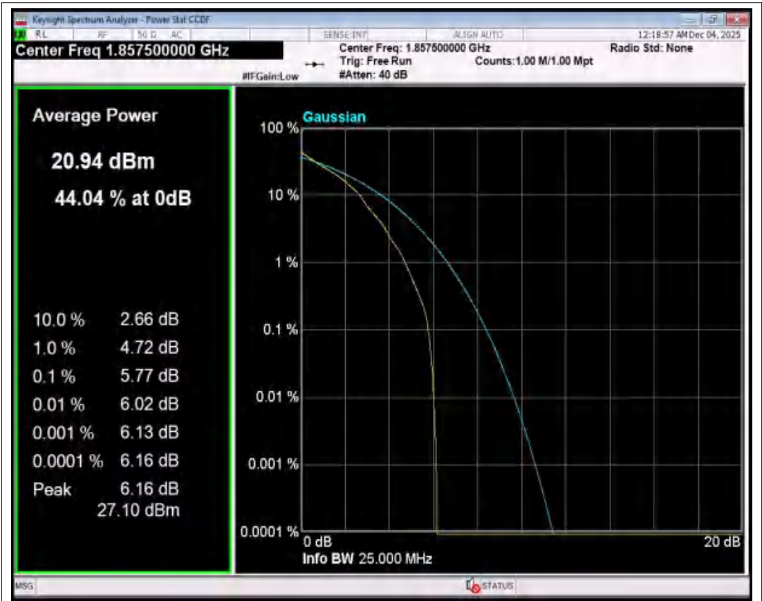
Band2 QPSK BW=15MHz Channel=18675 RB Size=1 Position=#0 NVNT
