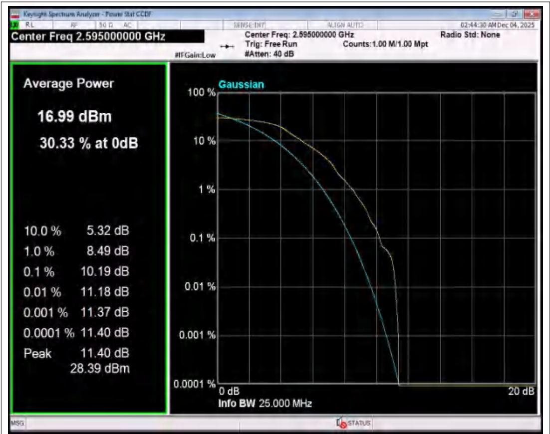
Band38 QPSK BW=15MHz Channel=38000 RB Size=1 Position=#0 NVNT
