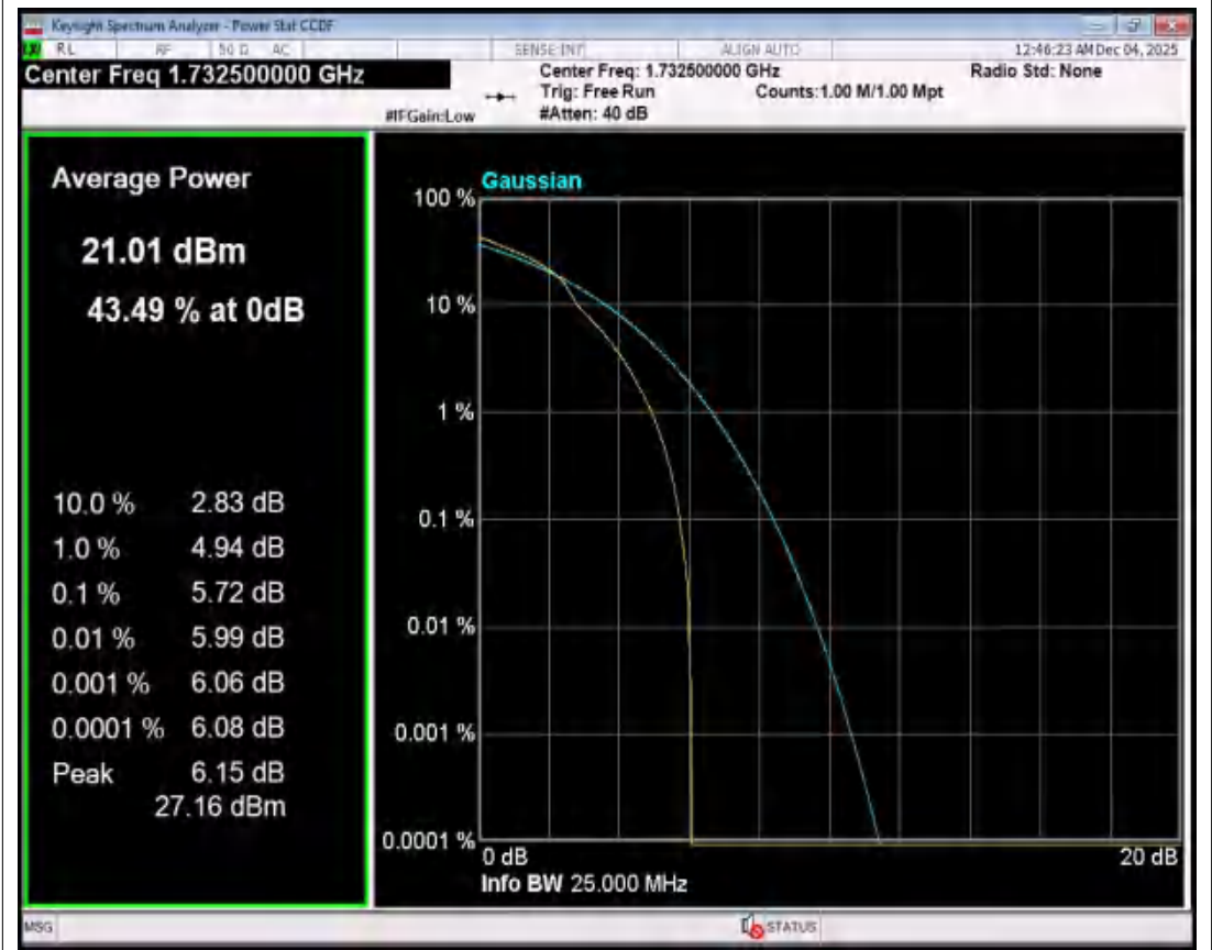
Band4 16QAM BW=5MHz Channel=20175 RB Size=1 Position=#0 NVNT
