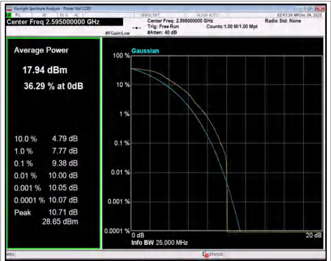
Band38 QPSK BW=5MHz Channel=38000 RB Size=1 Position=#0 NVNT
