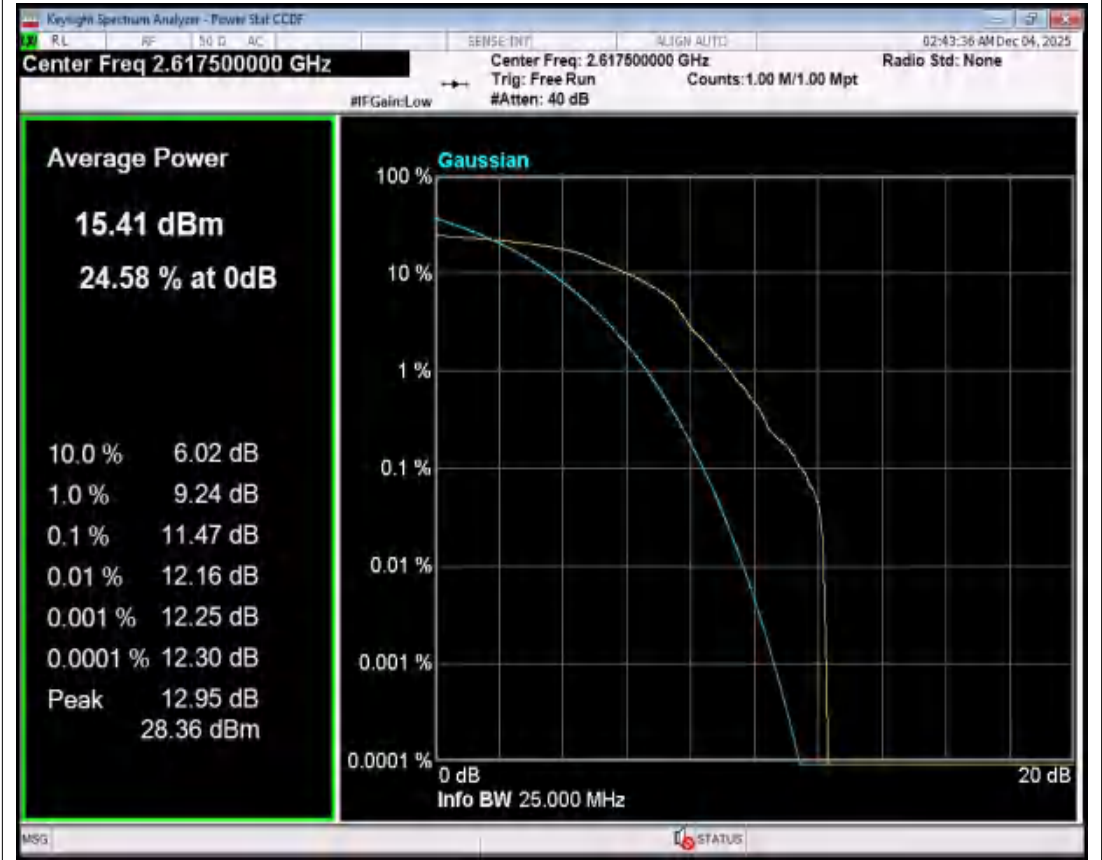
Band38 16QAM BW=5MHz Channel=38225 RB Size=1 Position=#0 NVNT
