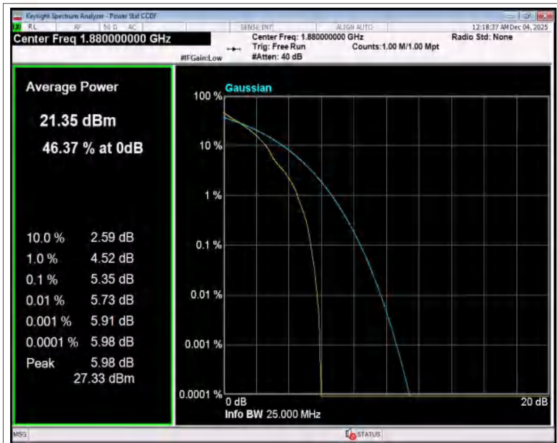
Band2 QPSK BW=10MHz Channel=18900 RB Size=1 Position=#0 NVNT
