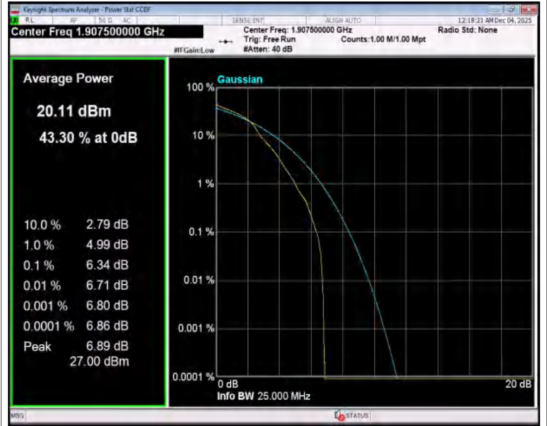
Band2 16QAM BW=5MHz Channel=19175 RB Size=1 Position=#0 NVNT
