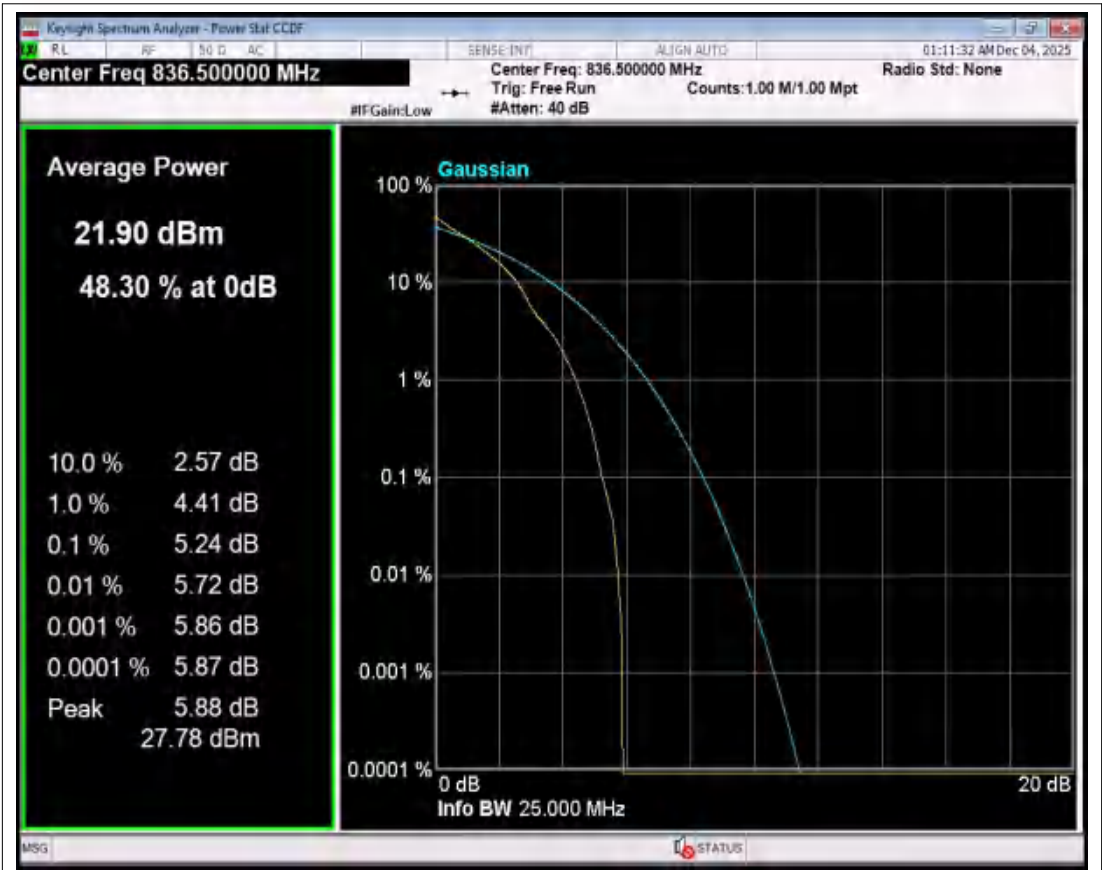
Band5 QPSK BW=1.4MHz Channel=20525 RB Size=1 Position=#0 NVNT
