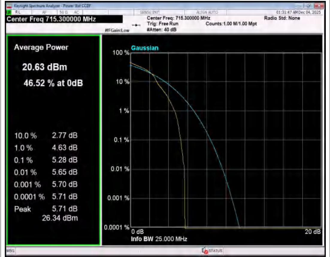
Band12 16QAM BW=1.4MHz Channel=23173 RB Size=1 Position=#0 NVNT
