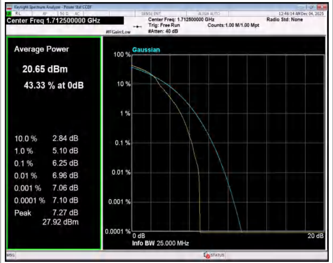
Band4 16QAM BW=5MHz Channel=19975 RB Size=1 Position=#0 NVNT
