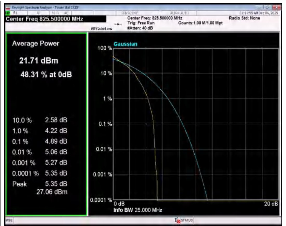
Band5 QPSK BW=3MHz Channel=20415 RB Size=1 Position=#0 NVNT
