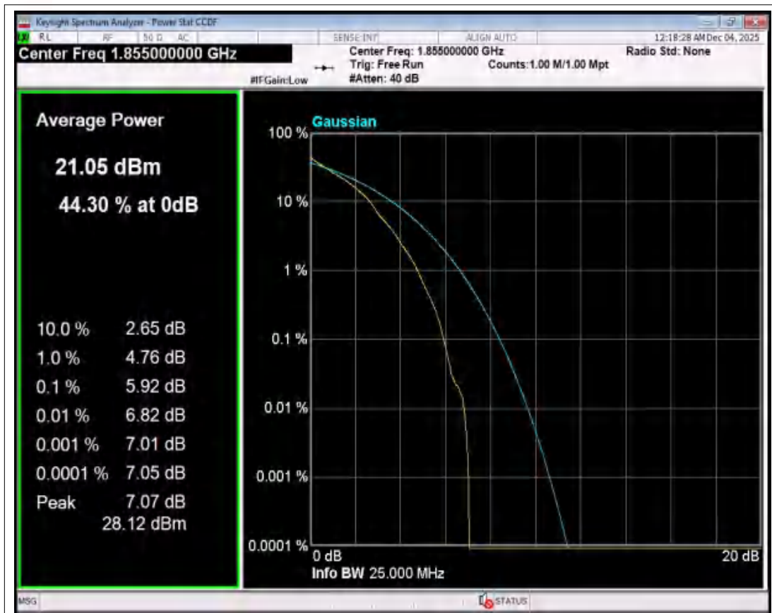
Band2 QPSK BW=10MHz Channel=18650 RB Size=1 Position=#0 NVNT
