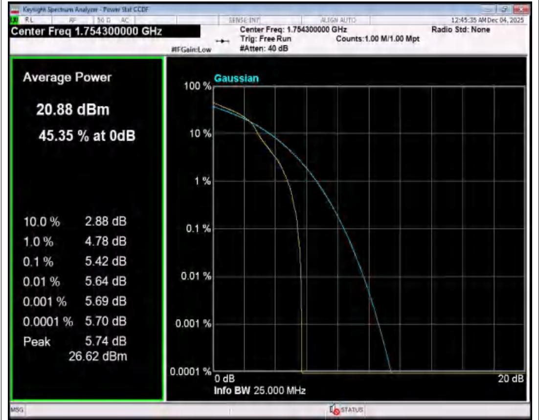
Band4 16QAM BW=1.4MHz Channel=20393 RB Size=1 Position=#0 NVNT
