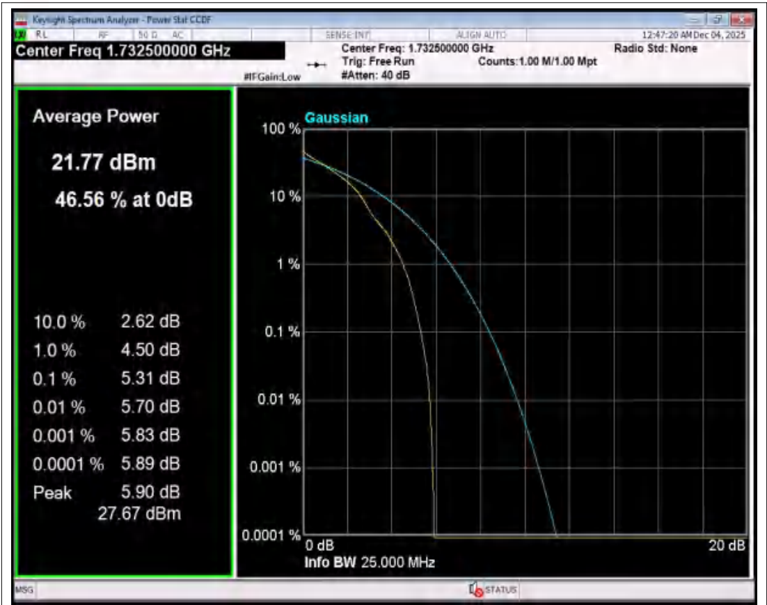
Band4 QPSK BW=15MHz Channel=20175 RB Size=1 Position=#0 NVNT
