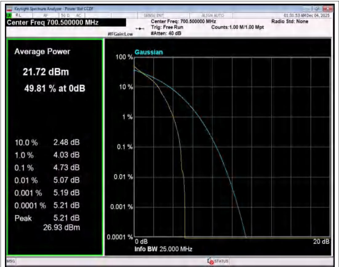
Band12 QPSK BW=3MHz Channel=23025 RB Size=1 Position=#0 NVNT
