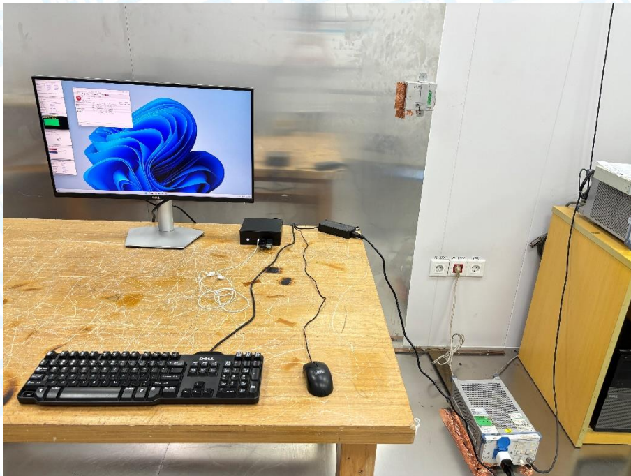
Photo of Setup for Conducted Emission
