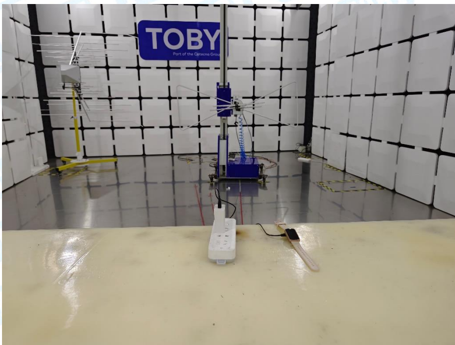
Photo of Setup for Radiated Emission (30MHz~1GHz)
