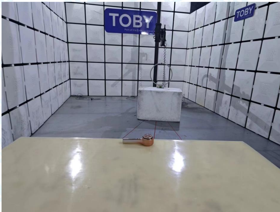
Radiated Emission Test Setup <30MHz
