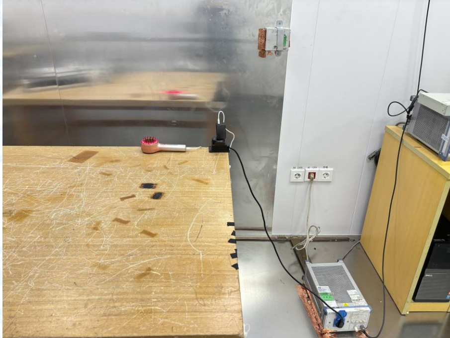
Photo of Setup for Conducted Emission
