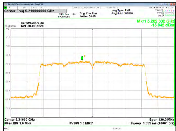
(802.11ac80) PSD plot on channel 42
