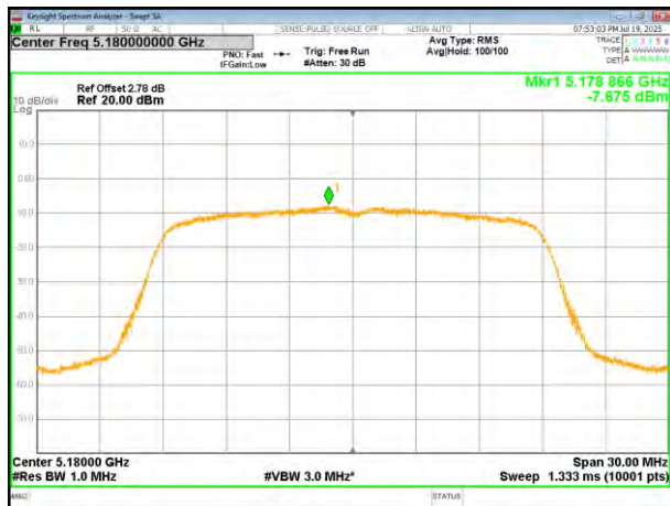
(802.11ac20) PSD plot on channel 36
