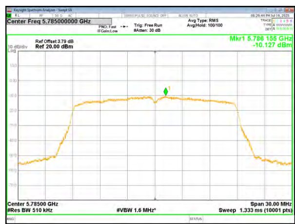
(802.11n20) PSD plot on channel 157
