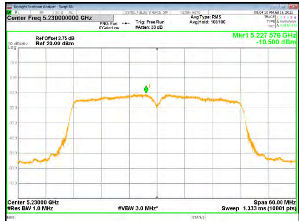
(802.11n40) PSD plot on channel 46
