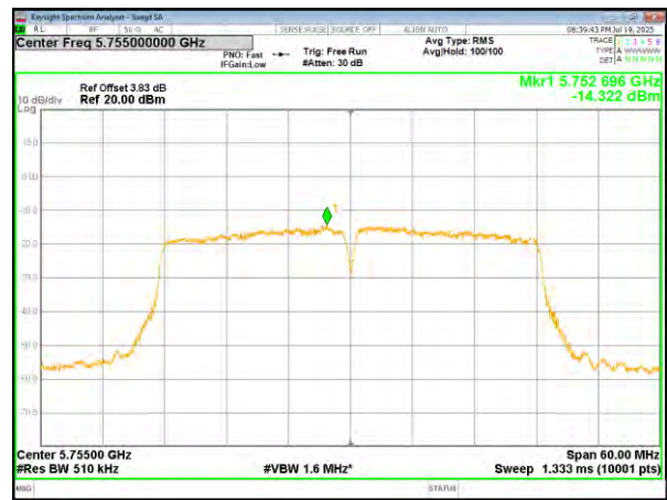
(802.11n40) PSD plot on channel 159
