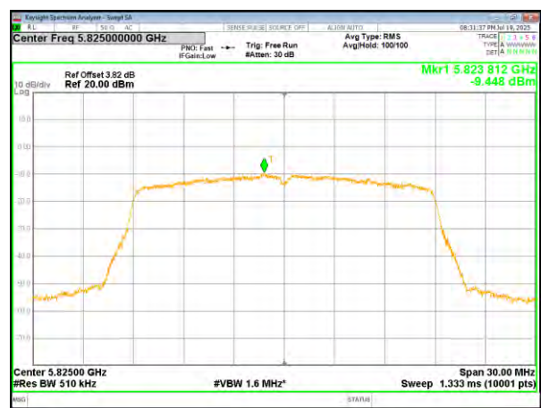
(802.11n20) PSD plot on channel 165
