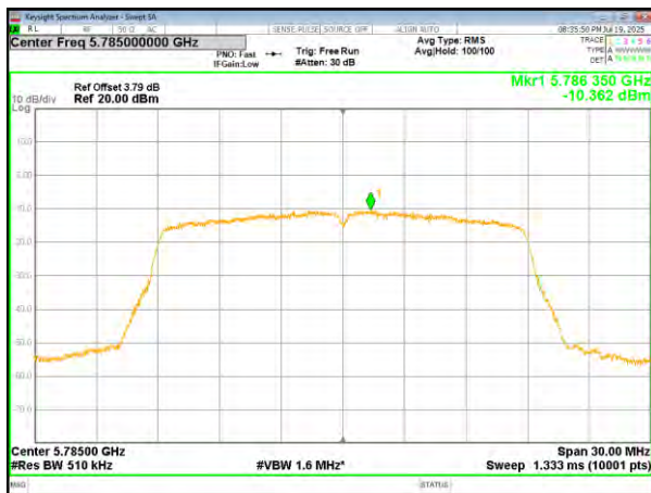
(802.11ac20) PSD plot on channel 157
