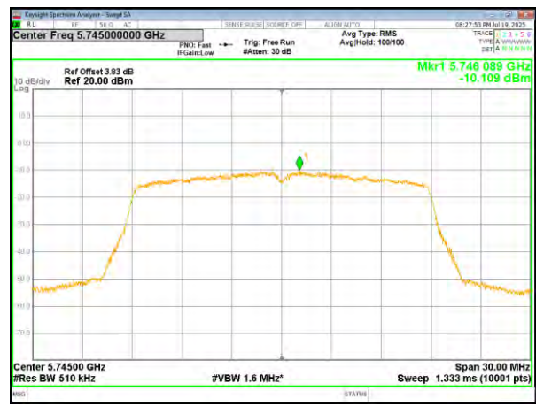
(802.11n20) PSD plot on channel 157
