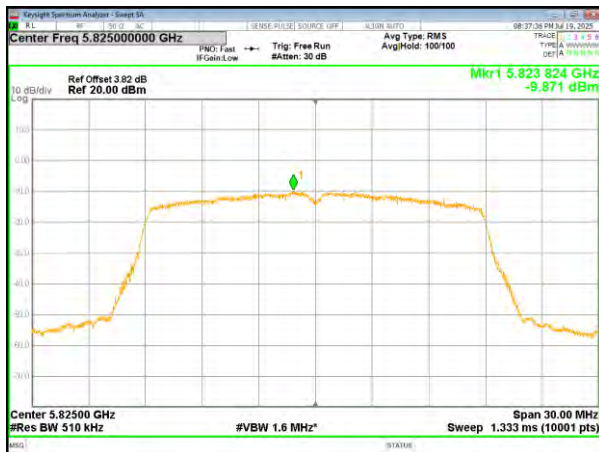
(802.11ac20) PSD plot on channel 165
