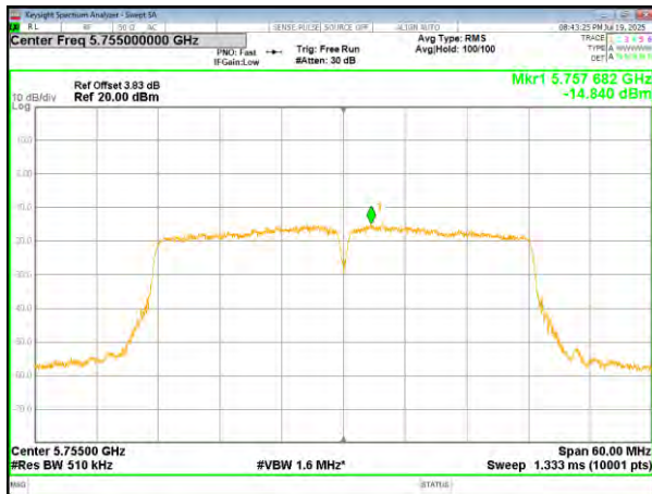
(802.11ac40) PSD plot on channel 159
