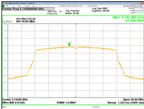
(802.11ac20) PSD plot on channel 157
