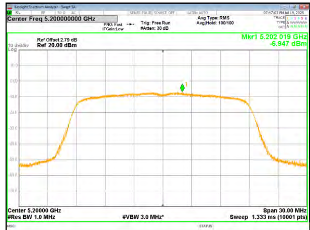
(802.11n20) PSD plot on channel 48
