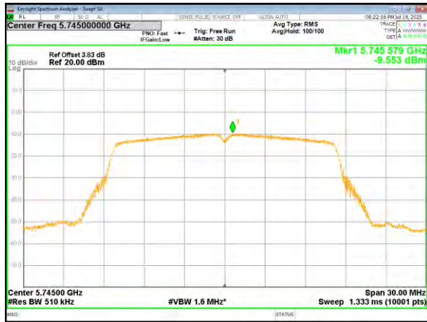
(802.11a) PSD plot on channel 157
