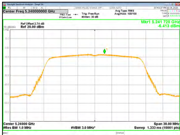
(802.11a) PSD plot on channel 48
