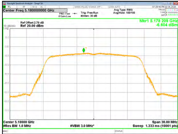
(802.11a) PSD plot on channel 36
