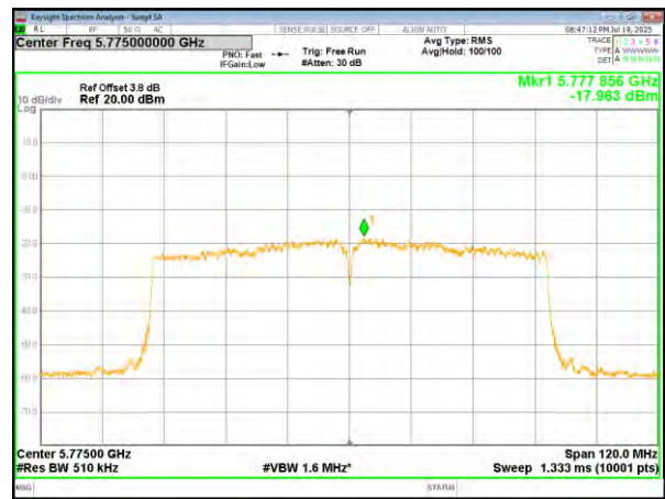
(802.11ac80) PSD plot on channel 155
