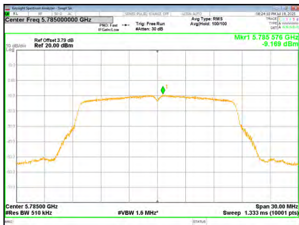
(802.11a) PSD plot on channel 157
