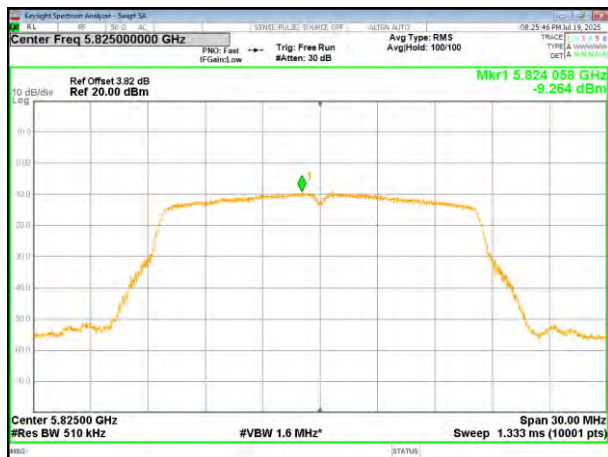
(802.11a) PSD plot on channel 165
