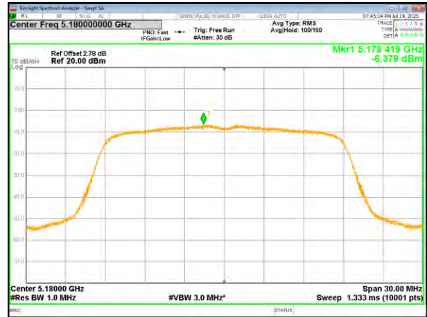
(802.11n20) PSD plot on channel 36
