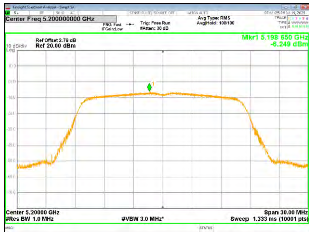
(802.11a) PSD plot on channel 48
