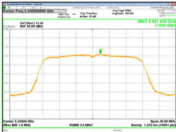
(802.11ac20) PSD plot on channel 48
