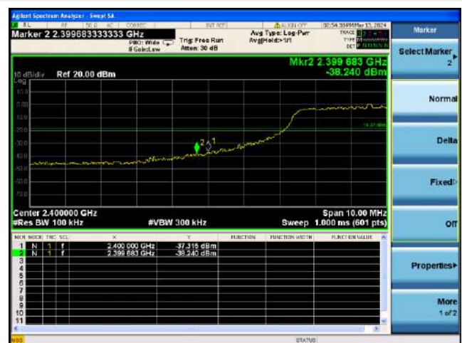
802.11ax-20 MHz(SU) LOW CHANNEL, BAND EDGE
