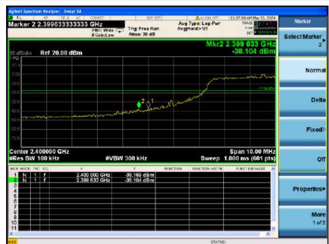
802.11ax-20 MHz(SU) LOW CHANNEL, BAND EDGE
