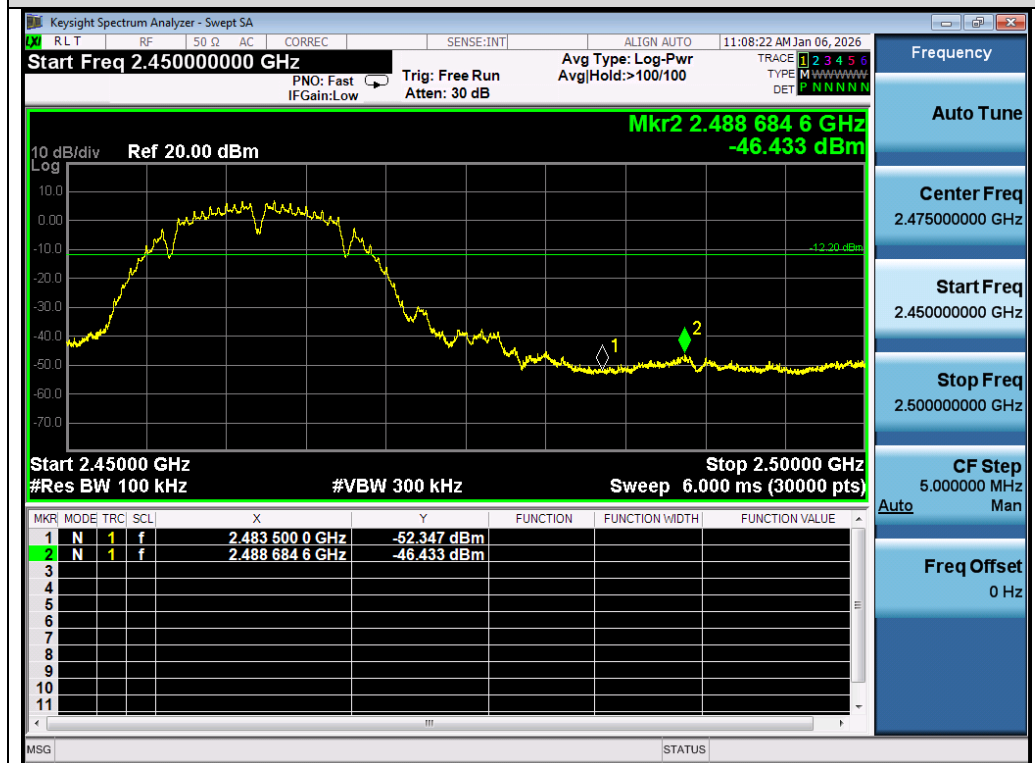
Test_Graph_802.11b_ANT1_2462_1Mbps_Higher Band Edge Emissions
