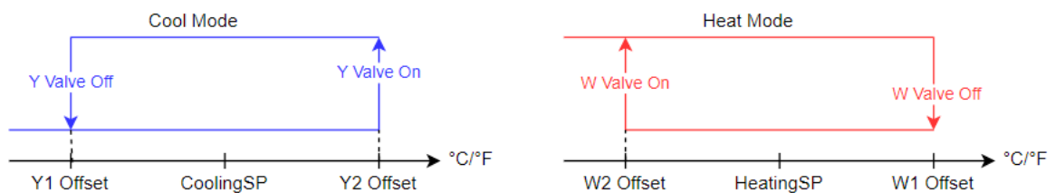
FIGURE 19: TWO PIPE COOLING AND HEATING MODE
