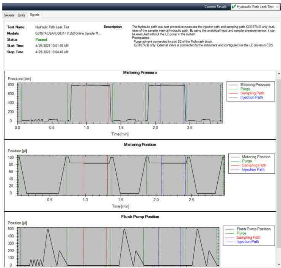
Figure 74 Hydraulic Path Leak Test passed
