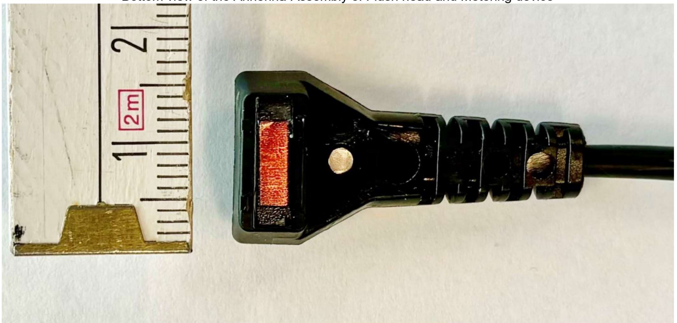
Bottom view of the Antenna-Assembly of Flush head and Metering device
