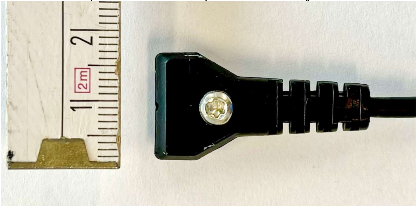
Top view of the Antenna-Assembly of Flush head and Metering device
