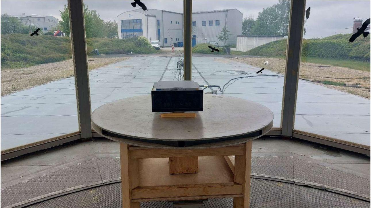
OATS 1 – Frequency Range: 30 MHz to 1 GHz
