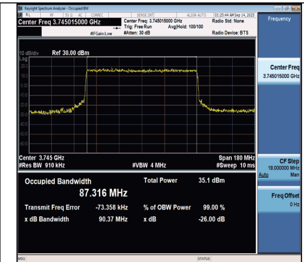
N77(3700-3980)-PC3-30-90-L-CP-64QAM-Outer_Full-Ant1-PASS
