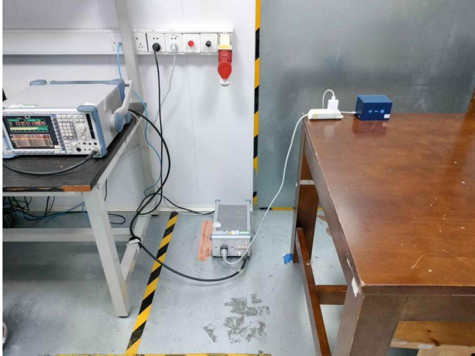
Conducted emissions at AC power line (150kHz-30MHz)
