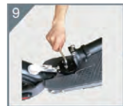
9. Tighten screw with a hexagonal wrench.
