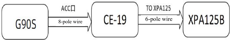
Schematic Diagram of Wiring between G90S and XPA125B
