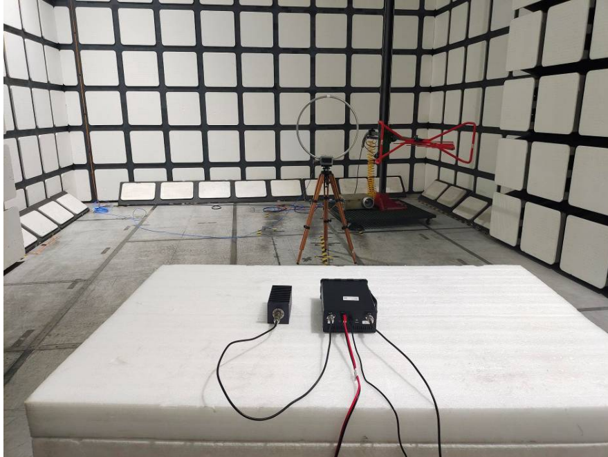
Radiated Emissions View (Below 30MHz)
