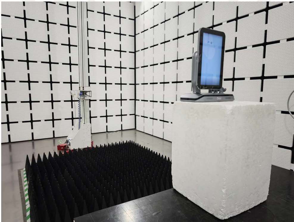
Spurious Radiation Emissions Test (> 1G)
