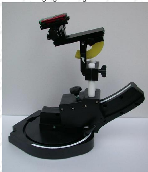
Device holder supplied by SPEAG
