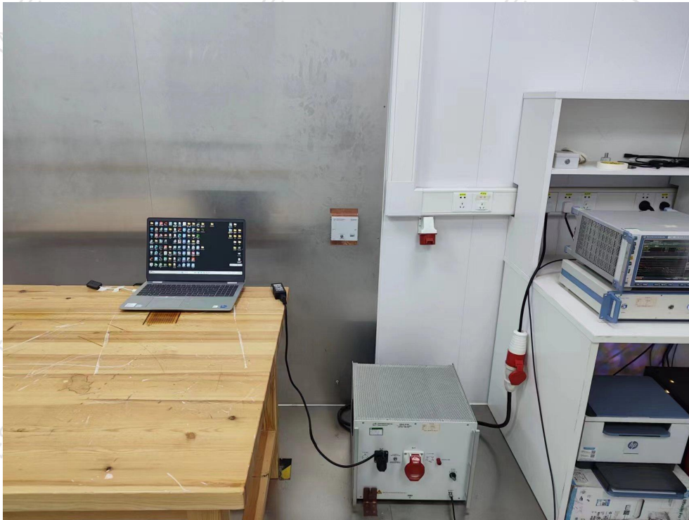
Photo of Conducted Emission Test
