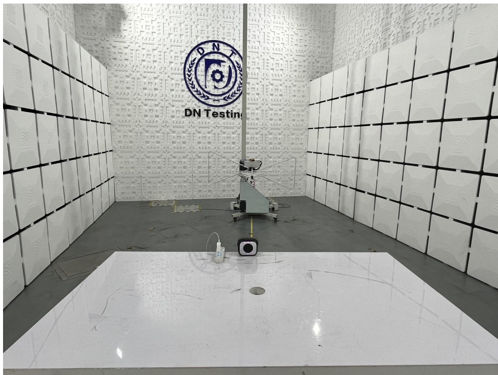
Radiated Emission Test View|(Below 1G)
