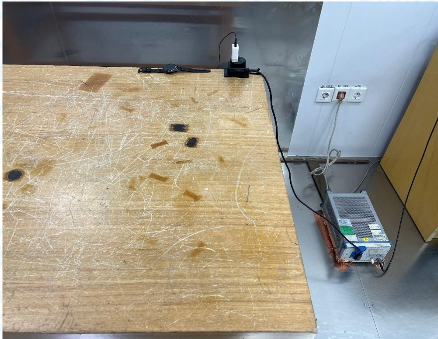
Photo of Setup for Radiated Emission (30MHz~1GHz)
