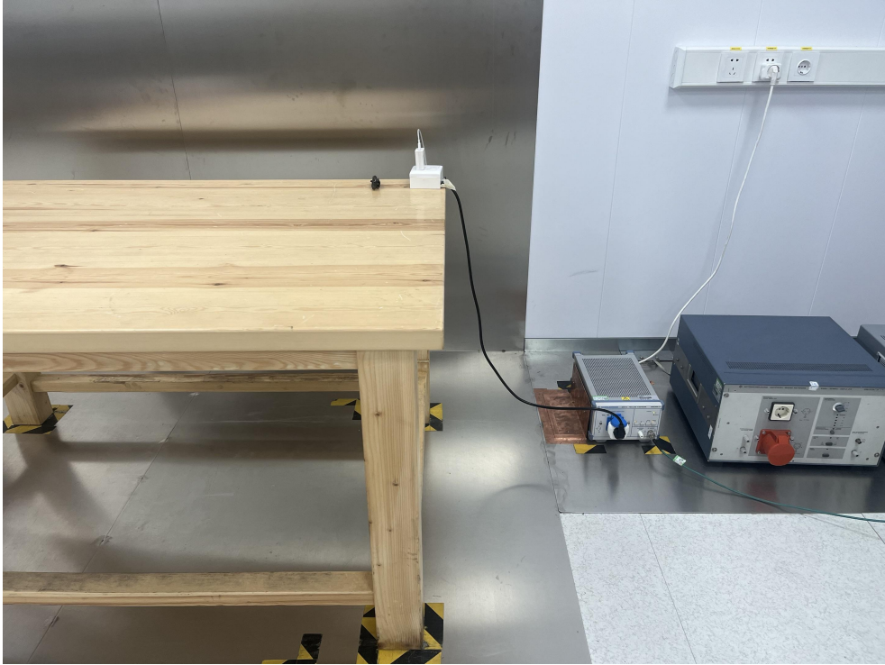
Radiated Emission Test View[(Below 1G)
