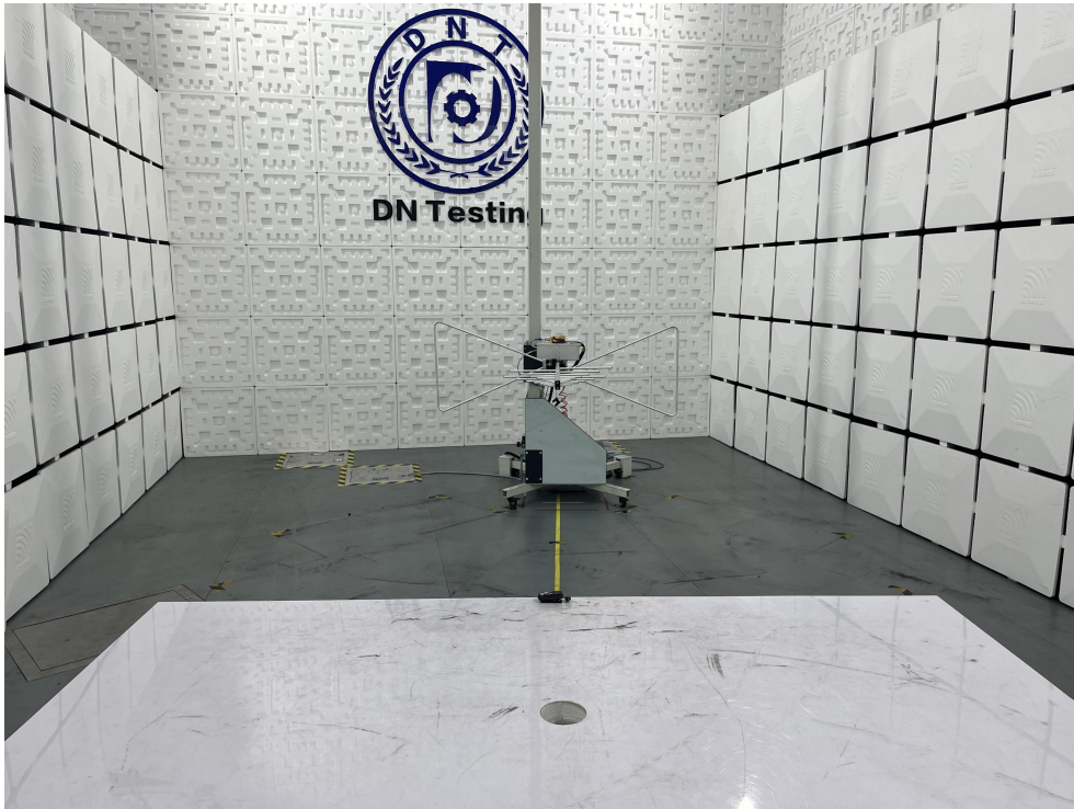
Radiated Emission Test View[(Below 1G)
