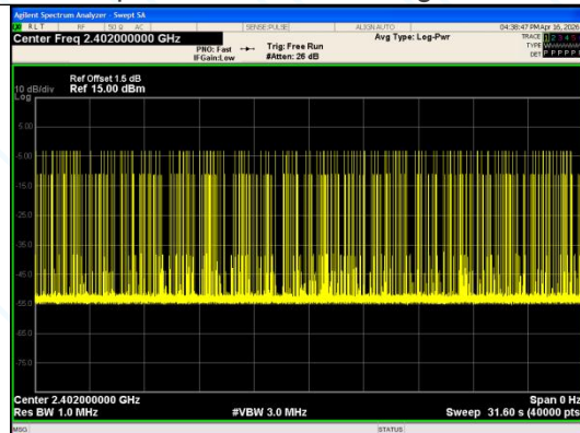
Number of Pulses in 31.6 seconds 8DPSK_3-DH3
