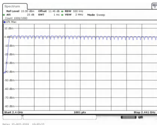
Low End Spectrum Channel Hopping Plot GFSK
