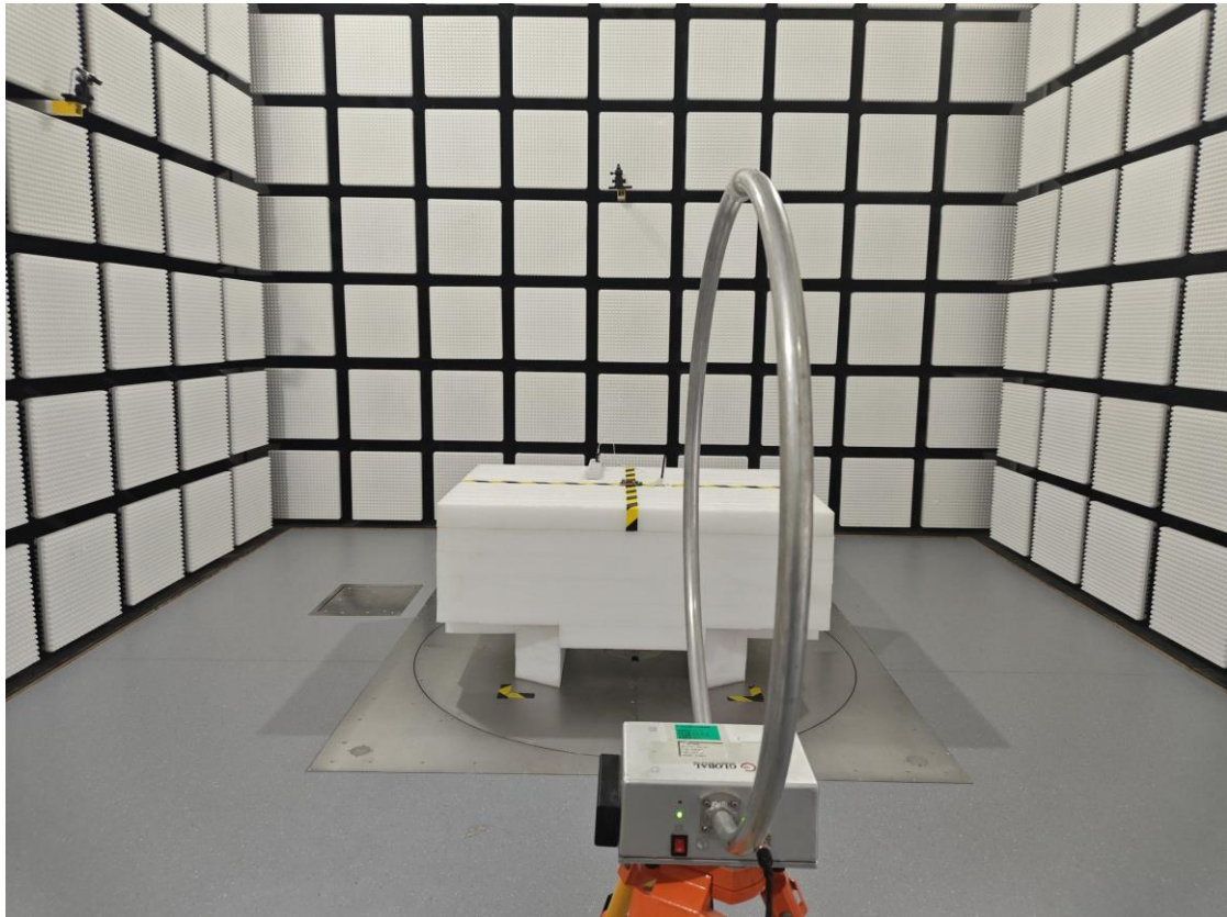
Radiated Emission 9 kHz-30 MHz Ground-parallel View
