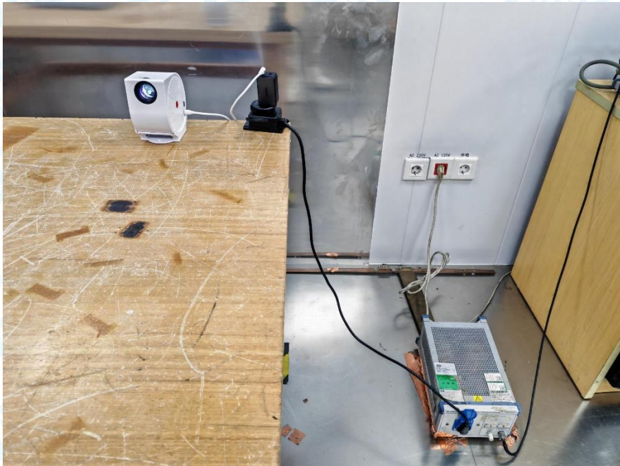
Photo of Setup for Radiated Emission (30MHz~1GHz)
