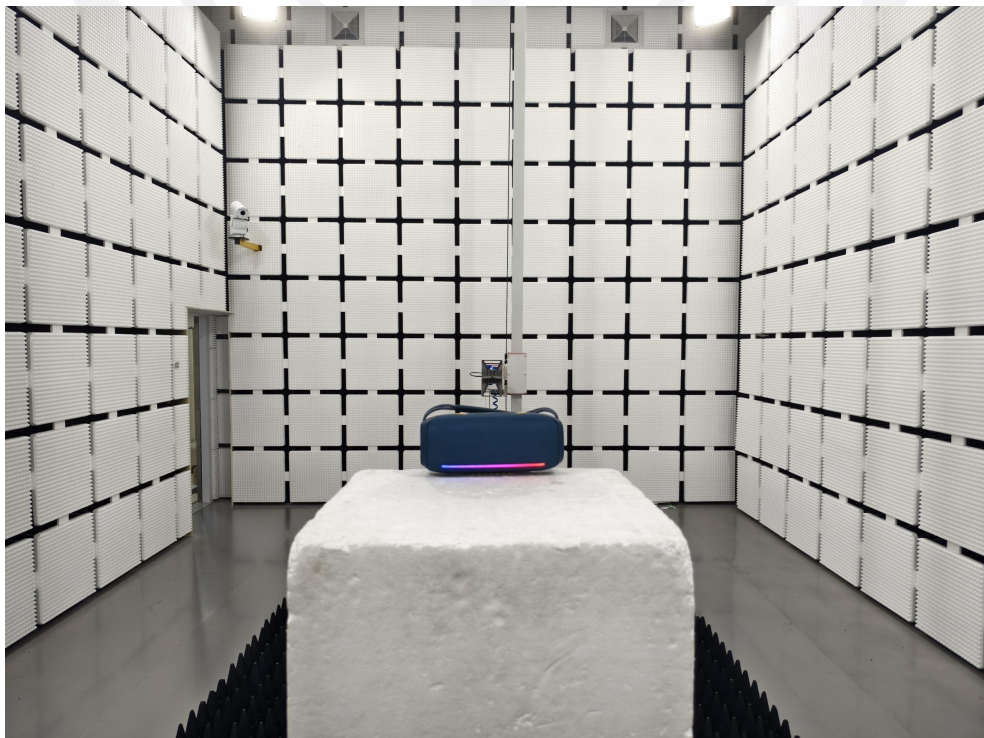
Spurious Radiation Emissions Test (> 1G)
